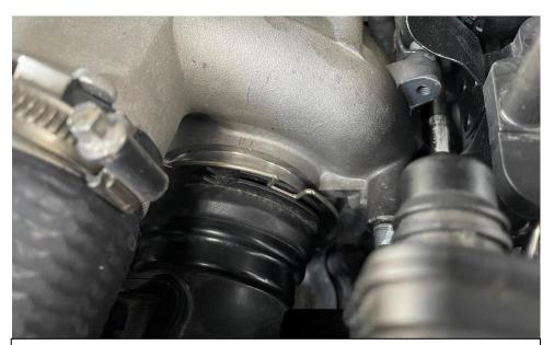
3. The inlets can be removed by pulling up the spring clips around the turbo flanges.
