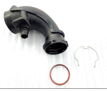
5. Remove the spring clip and the internal gasket from the inlets. Note the orientation of the gasket. It needs to go back into the carbon inlets in the same orientation.
