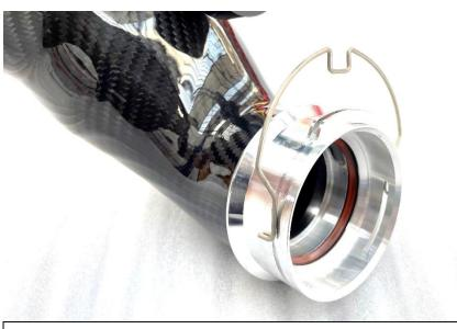
6. Insert the spring clip onto the machines flange with the top of the clip positioned over the raised section. Also insert the O-ring inside the flange as shown. The tapered face of the gasket should face the turbo.
