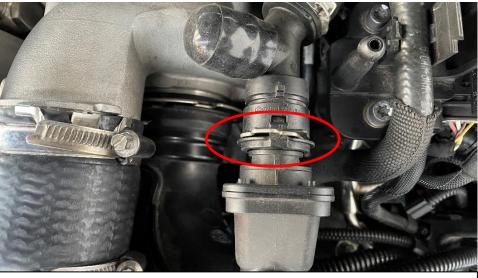
2. Pull up the spring clips holding the breather connectors to the inlets.
