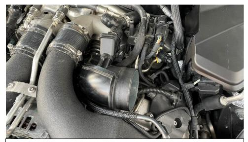
1. Start by removing the intake from the inlets.
