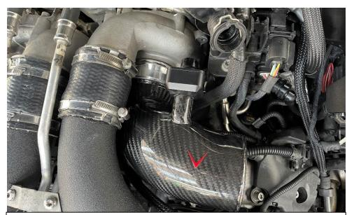
7. Push the inlets into place and secure with the clip. Connect the breather tube back into place and secure.
