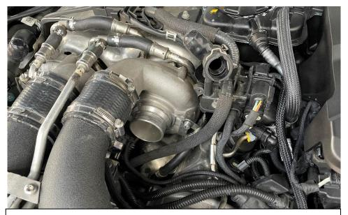
4. Remove the inlets from the turbos.
