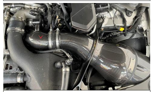
8. Now the intake can be installed back into place.
