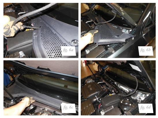
3. Unclip the hose from the cowl cover and remove both sections of cover from the vehicle (figs. 6a-6d).
