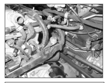
c. Install the aluminum spacer onto the mounting stud where the stock intake mounted.
