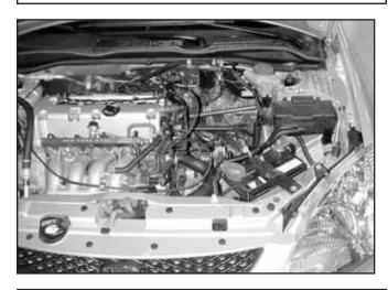
I. Factory air box system removed.
