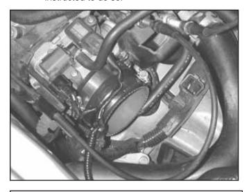
b. Install the 3" hose on to the throttle body using the #44 hose clamps. Check to see that the inside of the AEM® inlet pipe and air filter are clean and free from any foreign objects and/or obstructions.
