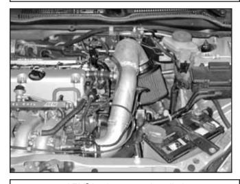
AEM® intake system installed
