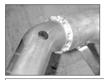
f. Install the supplied rubber grommet into the AEM® intake pipe.
