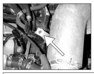
g. Slide the AEM® intake pipe into place under the throttle cables and above the radiator line. Align the mounting bracket with the mounting stud on top of the aluminum spacer previously installed. Install washer and serrated nut onto stud.
