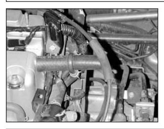
d. Where the stock rubber breather hoses were removed, replace them with the two supplied ¾" hoses. Replace this with the 1-¾" supplied high tensile breather hose. Then install the 2" breather hose onto the side that attaches to the AEM® intake pipe. Trim these hoses to fit. Use all 4 of the 1-1/16" hose clamps to secure
