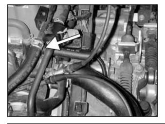
e. Install the provided 3/8" vacuum line onto the factory thermo valve.
