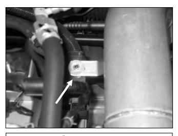
g. Slide the AEM<sup>®</sup> intake pipe into place under the throttle cables and above the radiator line. Align the mounting bracket with the mounting stud on top of the aluminum spacer previously installed. Install washer and serrated nut onto stud.
