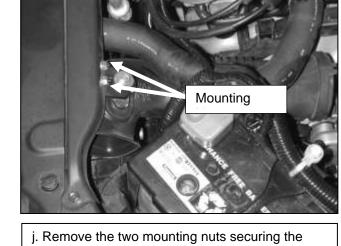
j. Remove the two mounting nuts securing the lower intake tube to the chassis. Then remove the inlet tube.
