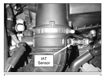
e. Remove the wiring harness from the rubber holds in the stock upper intake tube. Disconnect the inlet air temp sensor wiring harness. Loosen the spring clamp securing the inlet air temp sensor and remove. Set the inlet air temp sensor aside as it will be reinstalled on the AEM® intake system.
