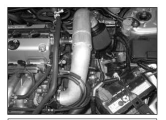
k. Check that the filter is not touching any part of the vehicle. Position the inlet pipe for best fitment. Be sure that the pipe or any other component is not in contact with any part of the vehicle. Tighten the hose clamps at the throttle body and silicone coupling. Tighten the nut on the mounting bracket.
