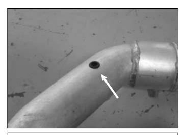
f. Install the supplied rubber grommet into the AEM® intake pipe.
