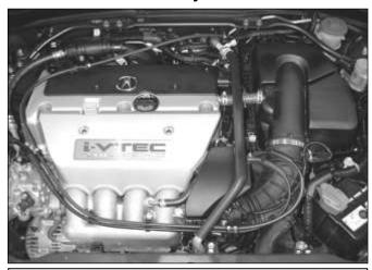
a. Factory air box configuration. Make note that there is one breather hose, one vacuum hose, and one Intake air temperature (IAT) sensor.
