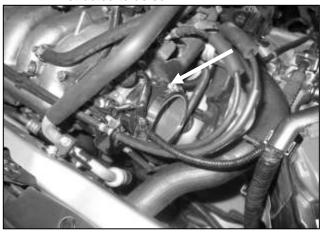
b. Install the 3" hose on to the throttle body using the #48 hose clamps. Check to see that the inside of the AEM<sup>®</sup> intake pipe and air filter are clean and free from any foreign objects and/or obstructions.
