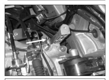
I. Remove the three bolts holding the stock air intake bracket to the transmission.
