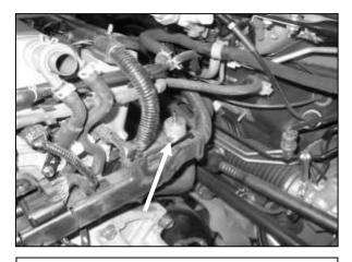
e. Install the aluminum spacer onto the mounting stud where the stock intake mounted.
