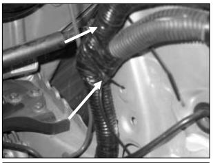
c. Clip off the zip tie holding the wire harness to the top of the shock tower. Use the supplied 11.25" zip tie to reattach the harness by snaking the zip tie through the metal support bracket on the shock tower. Use the supplied mounting zip tie to replace the upper zip tie previously clipped as shown. Remove excess.
