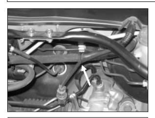
d. Zip tie rear electric line to insulated heater line as shown using supplied 6" zip tie. Cut off excess.
