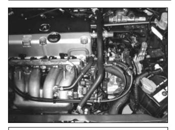
k. The factory air box system removed
