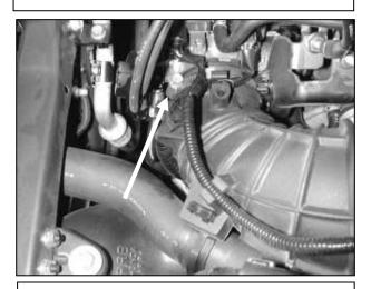
d. Remove the hose clamp securing the stock upper intake tube to the throttle body.
