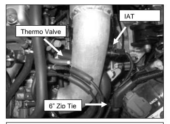
i. Attach the factory thermo valve line and install the IAT sensor into the rubber grommet. Plug the wiring harness into the IAT sensor. **Be careful not to damage the IAT sensor!** Use the supplied 6" zip tie to secure IAT sensor wire to battery wire.
