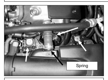
g. Loosen the spring clamp securing the crankcase breather tube and remove from the filter box. Remove the mounting bolt securing the filter box. Remove the mounting nut securing the filter box.
