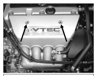
b. Remove the two mounting bolts securing the upper engine cover. Remove the engine cover.
