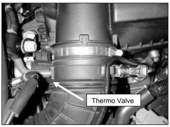
f. Remove the hose clamp securing the stock upper intake tube to the filter box. Remove the thermo valve hose. Remove the stock upper intake tube from the vehicle.
