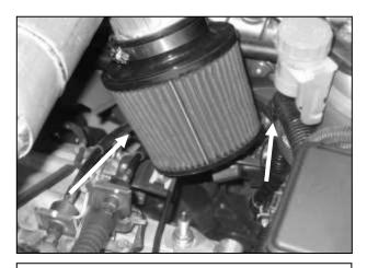
j. Install the AEM<sup>®</sup> air filter onto the end of the inlet tube. Push the air filter over the inlet pipe until the stop in the filter is reached. Then install the #56 hose clamp to secure the filter onto the inlet pipe. Once proper fitment is confirmed, tighten the hose clamp.
