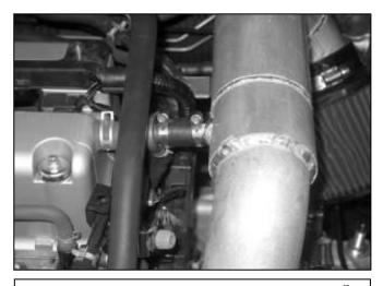
h. Slide the supplied breather hose onto the AEM<sup>®</sup> intake pipe and use the 1-1/16" hose clamps to secure. This hose should be trimmed to fit properly.
