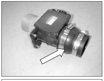
c. Attach the coupler to the MAF sensor using the provided hose clamps.
