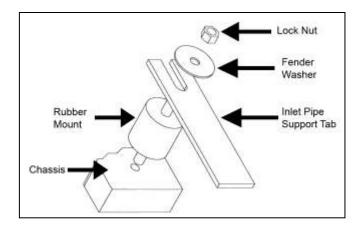
j. Proper installation of the rubber mount assembly.
