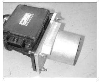
b. Attach the MAF sensor adapter to the MAF sensor using the supplied bolts and lock nuts.
