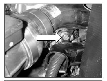
g. Place the intake pipe's bracket behind the specified stock plastic tab. Attach the bracket of the upper intake pipe to the engine, using the supplied 6mm bolt and washer as shown. Once secured, install the MAF sensor assembly onto the intake pipe; secure the side with the rubber coupler to the intake pipe.
