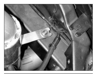
i. Install the rubber mount into the frame of the vehicle as shown. Align the lower intake pipe's bracket with the rubber mount and secure with a washer and lock nut. Do not completely tighten the lock nut. Refer to the diagram below to reference the proper installation of the rubber mount assembly.
