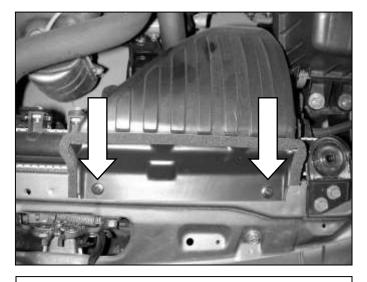
e. Release the air duct by removing the plastic rivets (Push in the center of the plastic rivet to remove).
