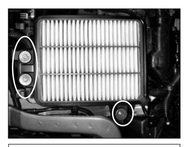
f. Loosen the three bolts holding down the lower air box assembly. Remove the air box and duct from the vehicle.
