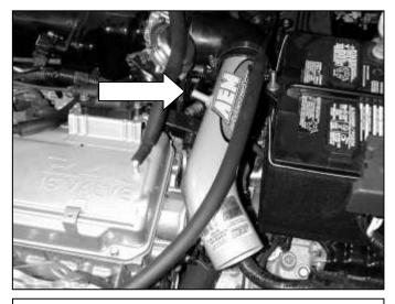
e. Insert the upper AEM<sup>®</sup> intake pipe into the rubber elbow. Ensure that the nipple of the intake pipe is facing the valve cover.
