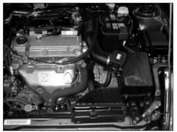
a. Factory air box system installed.
