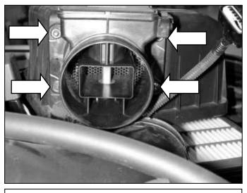
d. Loosen the four nuts that secure the MAF sensor to the air box. Carefully set the MAF sensor aside.
