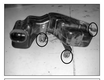
h. Loosen the three bolts that hold in the lower air box and remove it from the vehicle.
