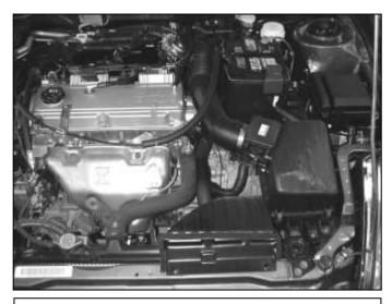
Factory air box system installed
