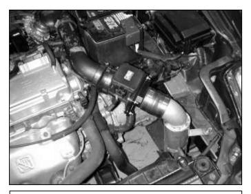
k. Install the air filter onto the lower end of the intake pipe. Once proper fitment and clearance is achieved secure the air filter with the supplied hose clamp.
