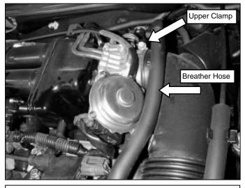
b. Pull the breather hose off the valve cover. Loosen the upper and lower hose clamps on the factory inlet tube.
