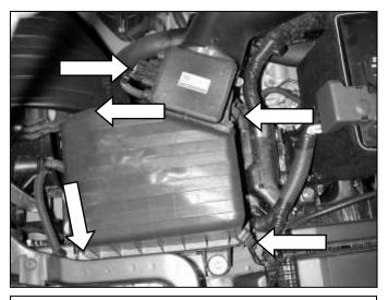
c. Unplug the MAF sensor. Remove the stock inlet tube. Release the four clamps on the air box and remove the upper air box from the vehicle.
