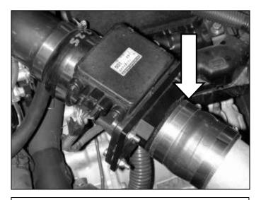
h. Plug the wiring harness into the MAF sensor. Install the straight coupler and hose clamps onto the upper section of the lower intake pipe. Guide the intake pipe into the engine bay, then attach the coupler to the MAF sensor. Secure the hose clamps, but do not completely tighten.
