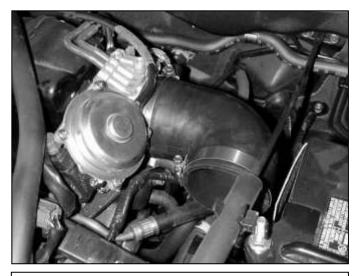
d. Place the rubber elbow with two hose clamps onto the throttle body. The longer end attaches to the throttle body.
