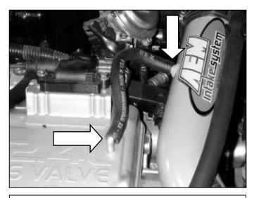
f. Install the supplied breather hose; secure both ends with the supplied  $\frac{3}{4}$ " hose clamps.
