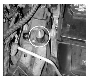
d. Thread the supplied rubber mount into the front hole where the aluminum bracket that mounted the IAC solenoid valve was located.
