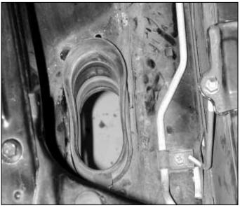
h. Remove the rubber sleeve from inside the fender.
