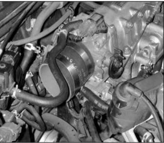
c. Install the 2.75" hose on to the throttle body using both #44 hose clamps. Check to see that the inside of the AEM<sup>®</sup> inlet pipe and air filter are clean and free from any foreign objects and/or obstructions.
