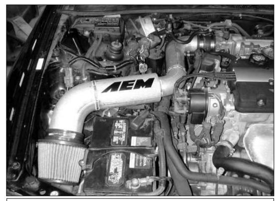
h. Check that the filter is not touching any part of the vehicle. Position the inlet pipe for best fitment. Be sure that the pipe or any other component is not in contact with any part of the vehicle. Tighten the hose clamps at the throttle body. Tighten the nut on the rubber mount. Check for proper hood clearance. Re-adjust pipe if necessary.
