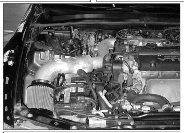
j. Check that the air filter is not touching any part of the vehicle. Position the inlet pipe for best fitment. Be sure that the pipe or any other component is not in contact with any part of the vehicle. Tighten the hose clamps at the throttle body. Tighten the nut on the rubber mount. Check for proper hood clearance. Readjust pipe if necessary.
