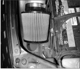
i. Next install the AEM<sup>®</sup> filter on to the end of the inlet tube. Push the air filter over the inlet pipe until it mates to the step inside the air filter inlet. Install the supplied #64 hose clamp to secure the filter onto the inlet pipe. Tighten the hose clamp after this is done.
