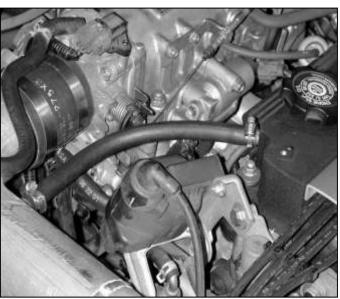
e. Install the  $\mathsf{AEM}^{\otimes}$  intake pipe into the 2.75" hose on the throttle body. The throttle body end is the end with the breather hose nipple.
