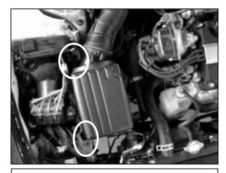
b. Remove the stock air box and intake system by loosening the hose clamp around the throttle body and removing the two airbox mounting bolts.
