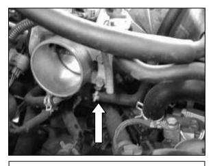
e. CAUTION: Ensure the engine is completely cool before removing the coolant hose, or hot coolant will escape from the cooling system and cause injury or damage. Be sure to capture any lost coolant in a clean container.
