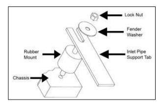
f. Proper installation of rubber mount assembly.
