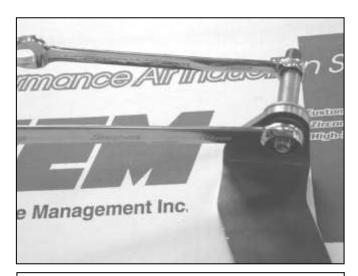
c. Install the factory mounting stud from step b on the supplied engine mount bracket, using the nylock nut and washer provided.
