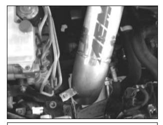
e. Align the tab on the intake pipe with the rubber mount. Install the 6mm nut and washer according to the diagram below. Do not tighten the nut.
