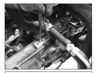
h. Install the spacer from the AEM<sup>®</sup> kit in place where the A/C line bracket was bolted. Install it with the pin inserted into small un-threaded hole on the bracket. It may be necessary to push the pin into the hole with a punch or similar tool. Make sure that the spacer is oriented with the threaded hole toward the A/C lines.
