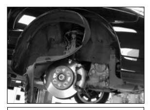
c. Remove the passenger side wheel. Partially remove the splash guard and tuck it out of the way.
