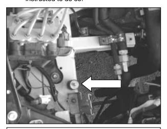
b. Install the rubber mount in the hole next to the radiator coolant reservoir bracket as shown in the picture.
