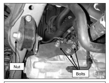
d. Using the supplied bolts and washers, install the AEM® engine mount on the transmission; torque the bolts to 61 ft-lb. Then replace the factory washer and nut on the mounting stud.
