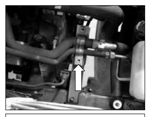
g. Remove the bolt holding the A/C line bracket in place.
