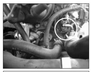
f. Remove the other end of the water bypass hose from the fitting on the engine. Install the other end of the 5/16" hose on to this fitting and secure both ends in place with 3/4" hose clamps.
