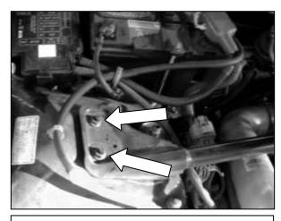
a. Remove the strut bar from the shock towers by removing the mounting nuts. Disconnect the PCV hose from the valve cover.
