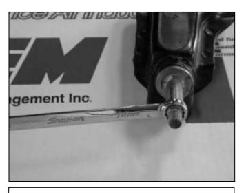
b. Using a 14 mm wrench, remove the mounting stud from the factory engine mount assembly. It may be necessary hold the bracket in a vice to do this.
