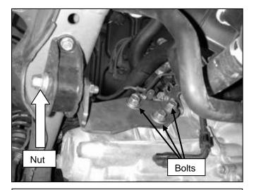
d. Using the supplied bolts and the factory washers, install the AEM® engine mount on the transmission, then replace the factory washer and nut on the mounting stud.
