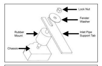
Proper installation of rubber mount assembly.
