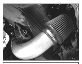
f. Install the air filter on the long end of the 4" diameter elbow. From underneath the vehicle, position the assembly so that the intake pipe and air filter **do not** make contact with the vehicle. Once proper fitment is achieved, secure the rubber mount's nut.
