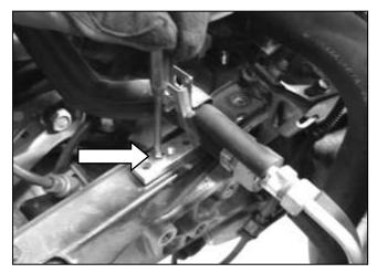
f. Install the spacer from the AEM® kit in place where the A/C line bracket was bolted. Install it with the pin inserted into small un-threaded hole on the bracket. It may be necessary to push the pin into the hole with a punch or similar tool. Make sure that the spacer is oriented with the threaded hole toward the A/C lines.
