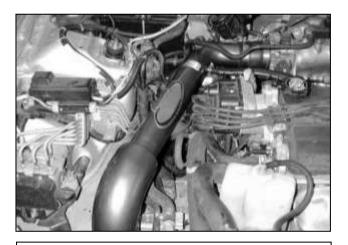
d. Insert the AEM<sup>®</sup> intake pipe in to the engine bay with the 2.5" end first, from the bottom of the vehicle. Slip the end of the intake pipe into the silicone coupler.
