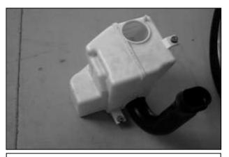
d. Remove the resonator from the cavity behind the front bumper (older models will be black).
