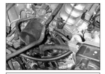
c. Insert the  $2.5^{\circ}$  x  $3.0^{\circ}$  coupler onto the throttle body (this is a tight fit). Slide the two #44 hose clamps over the end of the coupler.
