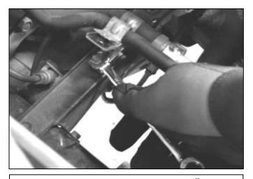
g. Using the M6 x 15mm bolt from the AEM® kit, bolt the spacer to the bracket.
