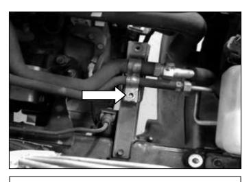
e. Remove the bolt holding the A/C line bracket in place.
