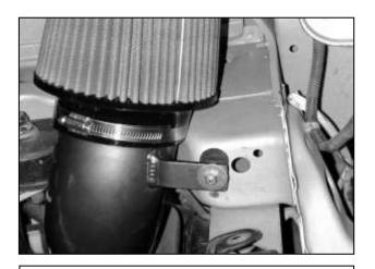
e. Align the tab on the intake pipe with the rubber mount. Install the 6mm nut and washer according to the diagram below. Do not tighten the nut.
