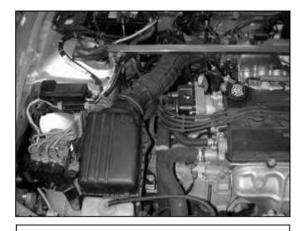
b. Remove the stock air box system by loosening the hose clamp around the throttle body and removing the two air box mounting bolts.
