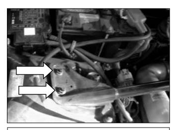
a. Remove the strut bar from the shock towers by removing the mounting nuts. Disconnect the PCV hose from the valve cover.
