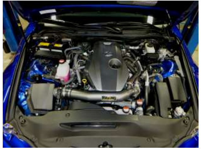
AEM INTAKE INSTALLED
