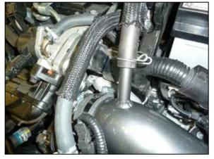
22. Connect the PCV hose to the AEM<sup>®</sup> intake tube and secure with the factory spring clamp.
