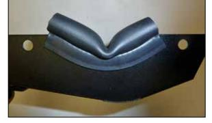
11. Install the 3.5" edge trim onto the bottom of the heat shield lid as shown.
