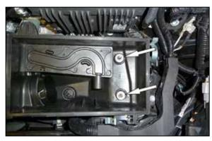
7. Remove the two bolts that secure the lower air filter housing and then remove the housing from the vehicle.
