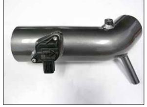
17. Remove the mass air sensor from the factory air filter housing and then install it into the AEM<sup>®</sup> intake tube and secure with the hardware provided.
