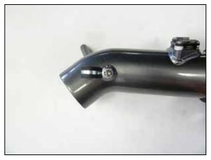
18. Install the provided loop clamp onto the AEM<sup>®</sup> intake tube and secure with the provided hardware.
