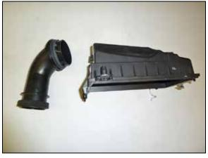
14. Remove the factory fresh air intake duct from the factory air filter housing.
