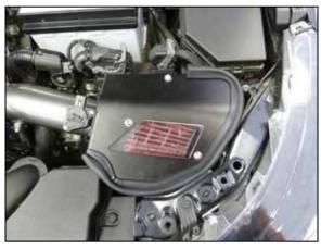
24. Install the heat shield lid and secure with the provided hardware.
