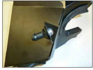
13. Install the mounting stud onto the heat shield using the provided hardware as shown.
