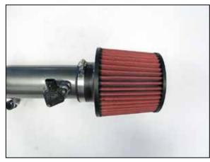
19. Install the AEM<sup>®</sup> air filter onto the intake tube and secure with the provided hardware.
