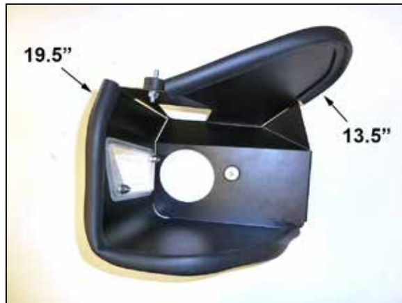
11. Install the provided edge trim onto the AEM® heat shield as shown.
