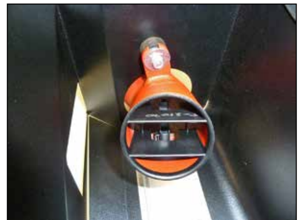
14. Install the intake tube through the heatshield and secure with the provided rubber mounted stud and hardware.
