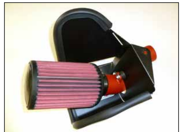
15. Install the AEM® air filter onto the intake tube and secure with the provided hose clamp.
