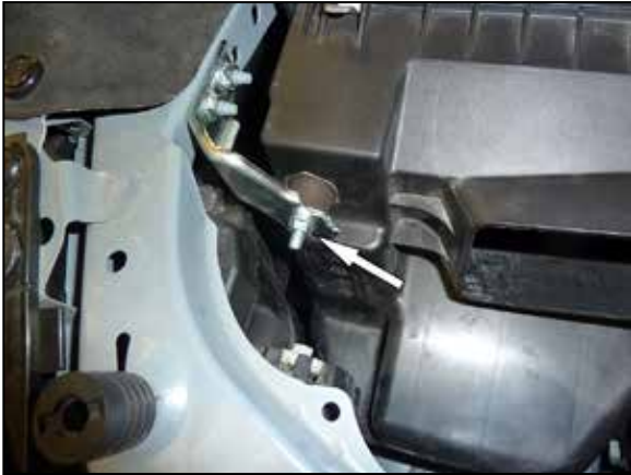
5. Remove the nut that secures the air filter housing to the inner fender bracket.
