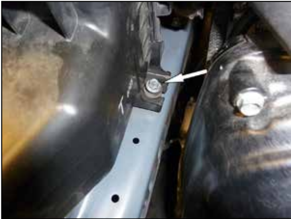
5. Remove the nut that secures the air filter housing to the inner fender bracket.
