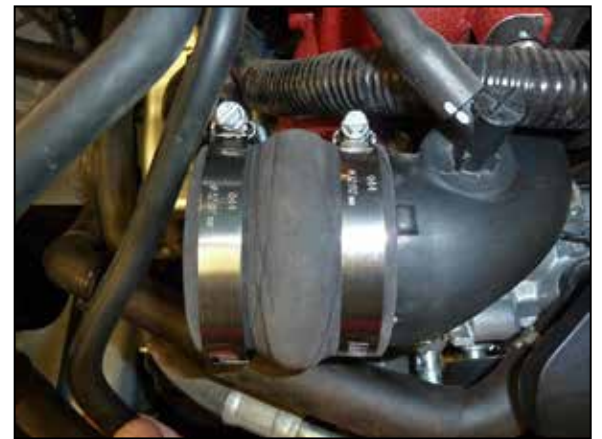
16. Install the provided hump coupler (08185) onto the turbo inlet and secure with the provided hose clamp.
