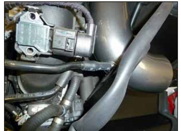
17. Connect the factory vent line to the fitting on the AEM® tube.
