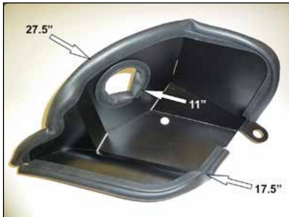
11. Install the edge trim onto the heat shield as shown.
