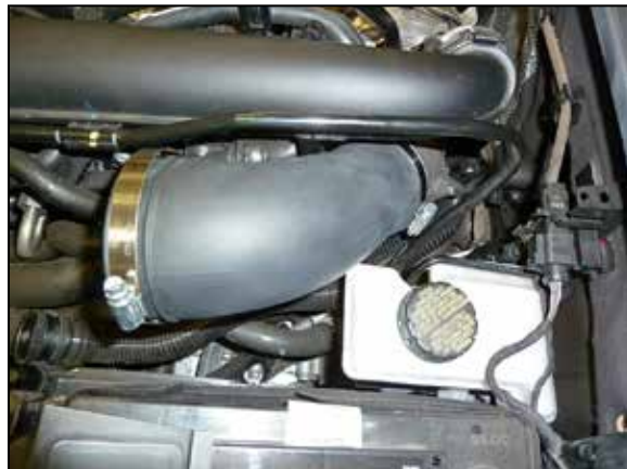
9. Install the provided angle coupler onto the turbo inlet and secure with the provided hose clamp.
