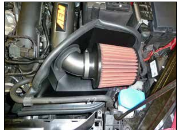
18. Install the AEM® air filter onto the intake tube and secure with the provided hose clamp.
