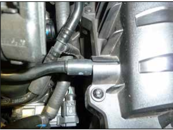
4. Disconnect the vent line from the air filter housing.
