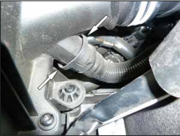
6. Squeeze the BOV quick release clamp and then disconnect the BOV hose from the factory air filter housing.
