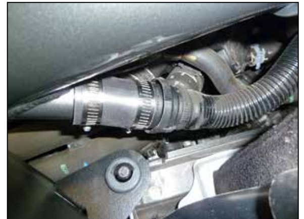
16. Connect the factory BOV hose to the quick disconnect fitting attached to the AEM® intake tube.
