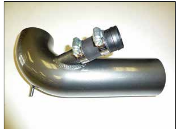
14. Install the provided BOV hose and quick connect fitting onto the AEM® tube as shown.
