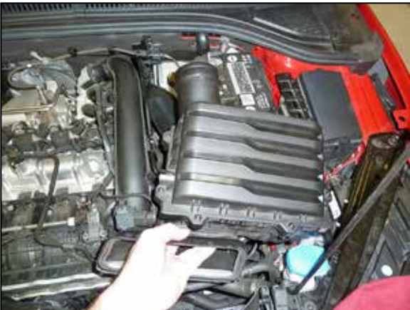
7. Pull the factory air filter housing up and remove it from the vehicle.
