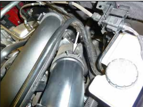
8. Release the spring clamp that secures the factory intake tube to the turbo inlet and then remove the tube from the vehicle.
