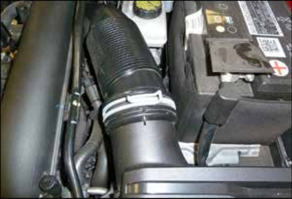
5. Release the clamp that secures the factory intake hose to the air filter housing and then disconnect the hose from the housing.
