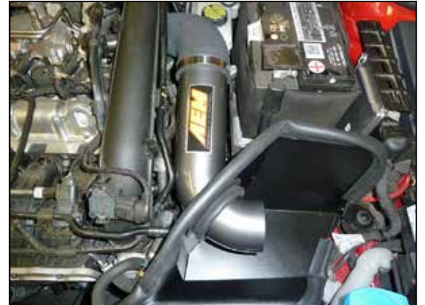
15. Install the AEM® tube into the coupler and heat shield as shown, Align the tube for best fit and secure with the provided hose clamps.
