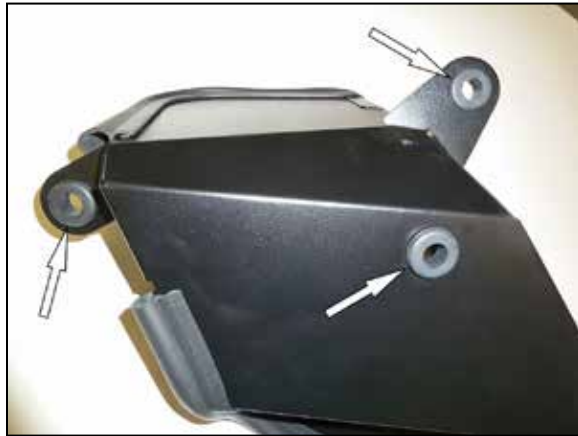
12. Install the mounting grommets into the heat shield as shown.
