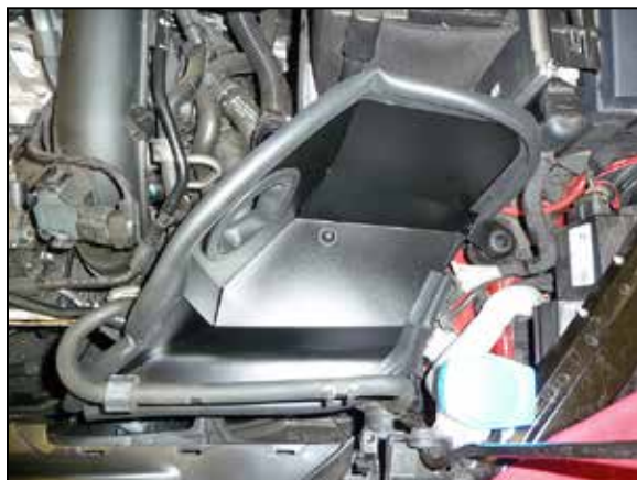
13. Install the heat shield onto the factory mounting studs as shown.
