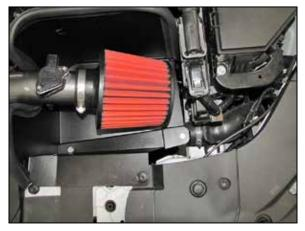
13. Install the AEM<sup>®</sup> air filter and secure with the provided hose clamp.
