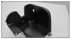
6. Install the provided edge trim onto the heat shield as shown, some trimming of the edge trim will be necessary.
