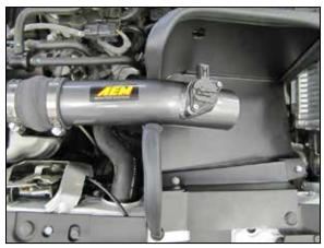
12. Install the AEM<sup>®</sup> intake tube into the coupler at the turbo inlet and then align the mounting stud with the hole in heat shield. Adjust the intake tube for best fit and then secure with the provided hardware and hose clamp.
