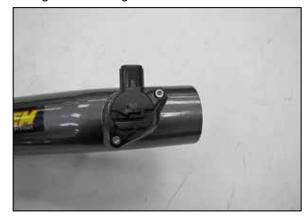
10. Remove the mass air sensor from the factory intake tube and install it into the AEM<sup>®</sup> intake tube and secure with the provided hardware.
