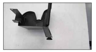
7. Remove the mounting grommet from the factory air filter housing and install it into the AEM<sup>®</sup> heat shield as shown.
