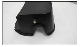
8. Install the rubber mounted stud onto the heat shield using the provided hardware.
