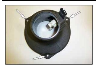
7. Install the provided spacers into the AEM<sup>®</sup> housing as shown.
