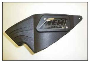
8. Install the AEM $^{\circ}$  badge into the filter housing and secure with the provided hardware.
