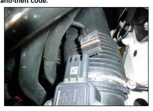
2. Disconnect the mass air sensor electrical connection. Loosen the hose clamp that secures the factory intake tube to the air filter housing.
