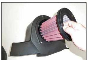
9. Install the AEM® air filter into the filter housing.
