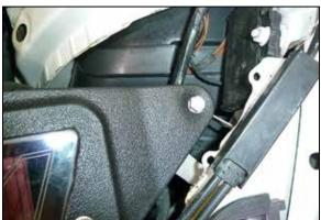
12. Install the remaining spacer into the air filter housing and then secure the housing with the provided hardware.
