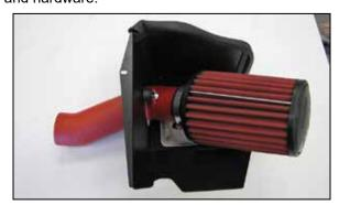
11. Install the AEM® air filter onto the intake tube and secure with the provided hose clamp.
