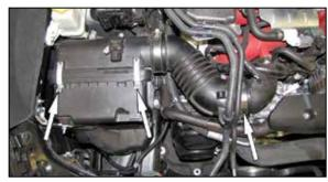
4. Loosen the hose clamp that secures the intake hose to the turbo inlet. Release the air filter housing clam shell clips and then remove the air filter clean side housing, intake hose and factory air filter from the vehicle.
