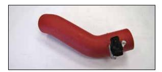
9. Remove the mass air sensor from factory housing and install it into the AEM® tube using the provided hardware.
