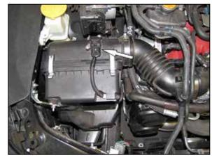
3. Disconnect the mass air sensor electrical connection and unclip the wiring harness from the air filter housing.
