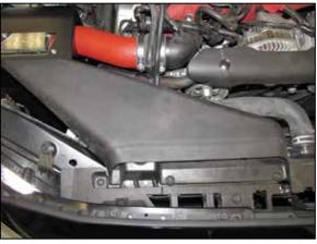
14. Install the fresh air duct and secure with the factory hardware.
