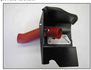
10. Install the intake tube through the heatshield and secure with the provided rubber mounted stud and hardware.
