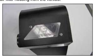
7. Install the AEM® window into the heat shield using the provided hardware and backing plate.
