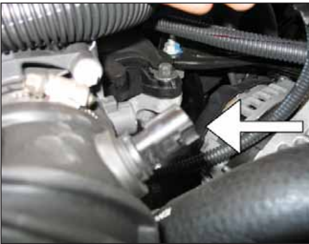
c. Locate the IAT sensor on the inlet tube and release the wire harness connector from the IAT sensor.
