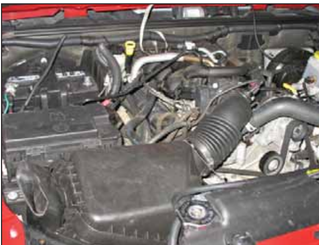
Factory air box system installed
