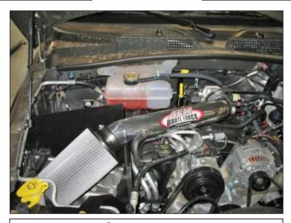
AEM® intake system installed
