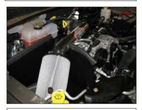
m. Attach the air filter and secure with a hose clamp once properly aligned. Attach the rubber edge trim to the top of the heat shield as shown.
