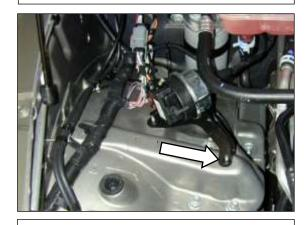
g. Loosen and remove the mounting nut. This nut will be reused if your vehicle has cruise control. If your vehicle is not equipped with cruise control, then use the provided M6 nut.
