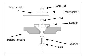
d. Diagram of the spacer assembly.
