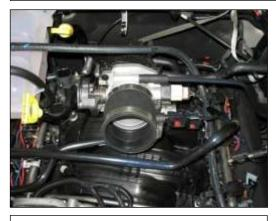
f. Attach the coupler as shown. Secure with #52 hose clamp on the throttle body and #48 on the open end. Reattach the IAT sensor harness to the IAT sensor.
