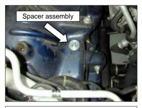
c. Mount the spacer assembly in the lower rubber mount left by the bottom of the airbox. The spacer assembly consists of the following: bolt, washer, spacers and nuts. Refer to the diagram on next page.
