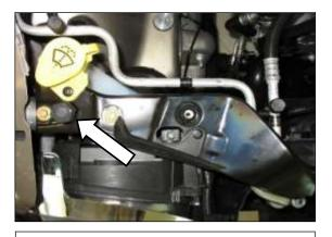
e. Remove the bolt, it will be reused in a later step.
