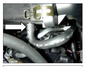
b. Disconnect the crankcase breather hose from the airbox. Remove the airbox by pulling straight up.
