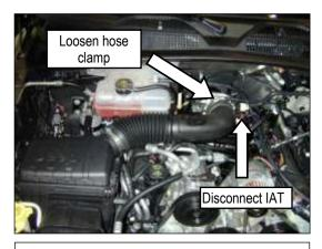
a. Loosen the hose clamp at the throttle body. Disconnect the IAT (Inlet Air Temperature) sensor harness connector. Push out the clip on the IAT to release.
