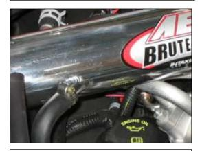
I. Rotate the breather hose 90° clockwise. Reattach the crankcase breather hose. Secure with the provided hose clamp.
