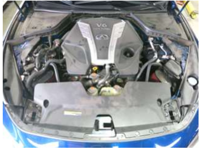
AEM INTAKE INSTALLED
