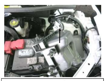
g. Pull up on the air box to release it from its grommets, disconnect the coupler, and turn the box on its side as shown to access the next wire tie. Release the harness from the air box and remove the air box from the engine bay.
