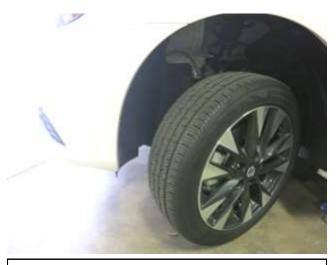
I. Lift the front of the car with a jack and turn the wheels to the left. **Note: Support car with jack stands once lifted.**
