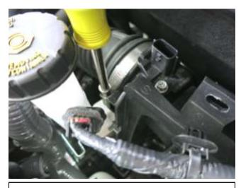
f. Loosen the hose clamp securing the factory coupler to the air box.
