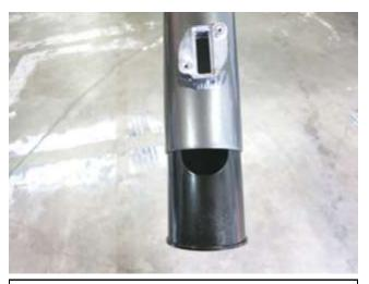
a. Align the hole in the venturi insert with the MAF pad as show and fully insert into the lower intake tube. **Note:** The venturi insert is necessary for proper engine function and performance.
