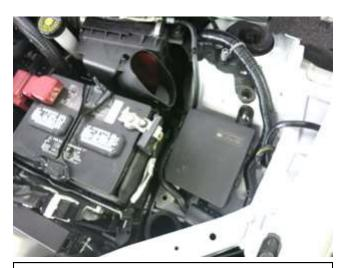
b. Lift the resonator duct up and out of the engine bay. Pull gently to release it from the grommet.
