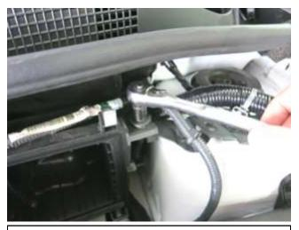
d. Remove the bolt securing the air box to the metal bracket.
