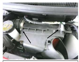
c. Unlatch the two clips on the air box and remove the forward section of the air box and the air filter from the engine bay.
