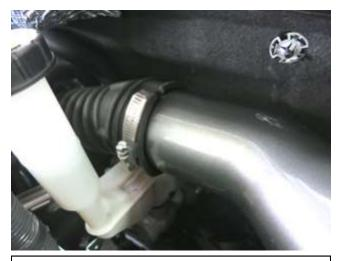
c. Connect the upper intake tube to the factory coupler. Soapy water can be used to help installation. Tighten this hose clamp at this time.
