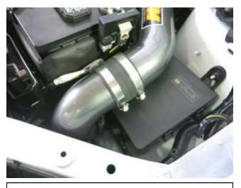
f. Bring the lower intake tube into the engine bay from under the fender well area and insert it into the coupler. Use care not to scratch the finish on your new intake tube. Masking tape can be used on the sharp edge of the core support if necessary. Do not fully tighten the lower hose clamp at this time.
