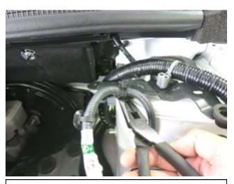
h. Release the final wire tie from the metal bracket as show and move the MAF harness down and out of the way.
