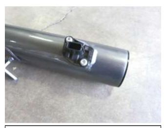
b. Install the MAF sensor into the lower intake tube using the screws removed in step 2p.
