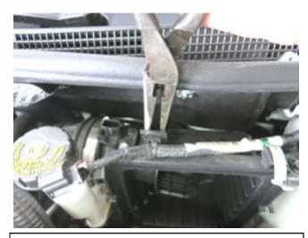
e. Disconnect the Mass Air Flow (MAF) sensor harness. Release the harness from the air box using pliers as shown.
