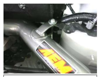
d. Loosely secure the upper intake tube to the factory metal bracket using the provided bolt and washer.
