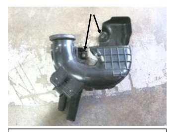
k. The positions of the two bolts from step 2j as seen from the front of the car are shown by the arrows. The left-hand side bolt will require a short extension. Allow the resonator to fall to the bottom of the bumper area once both bolts are removed.
