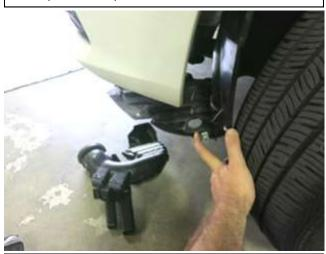
o. Pull back the inner fender liner to remove the stock intake resonator. **Note: Do not discard any of your stock equipment.**
