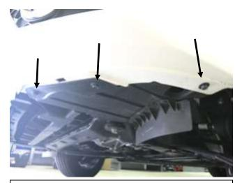
n. Remove the three bolts securing the front of the inner fender liner.
