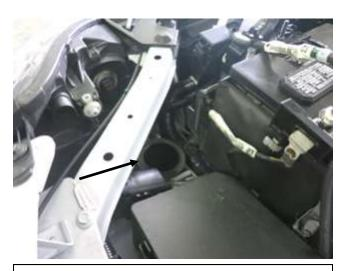
j. Use the next picture to help in removal of the intake resonator indicated in this step. Both bolts are accessible from above using a ratchet, socket, and extension.
