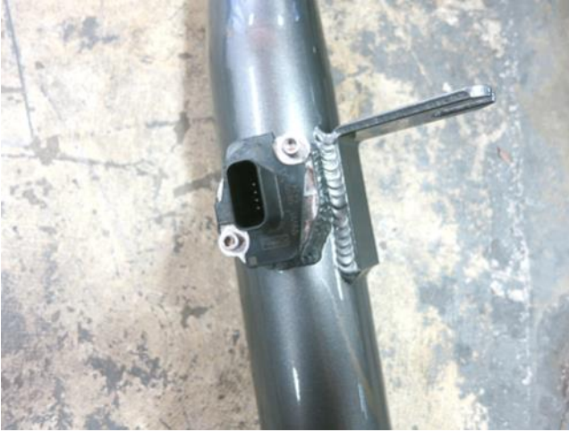
a. Install the IAT sensor into your AEM intake tube using the provided hardware.
