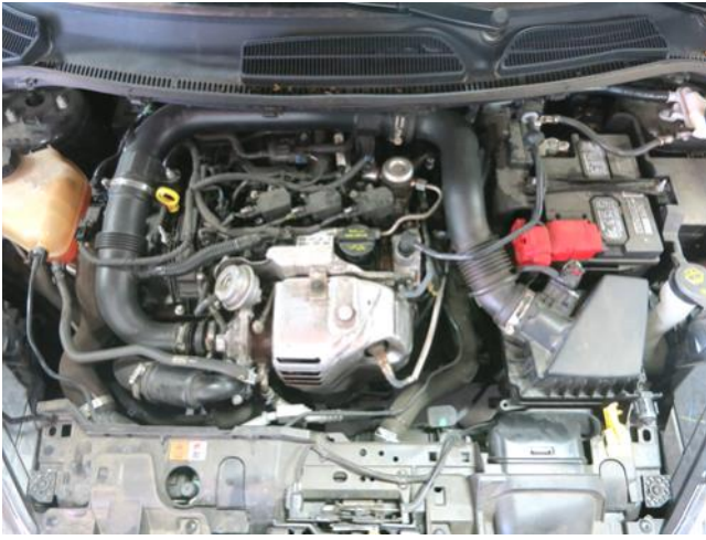
STOCK INTAKE INSTALLED
