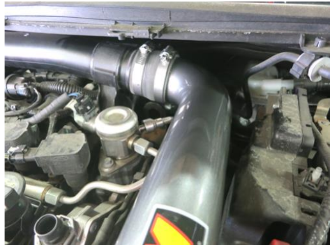
d. Lower your AEM intake tube into the engine bay and insert the end into the coupler. Do not tighten the hose clamp at this time.
