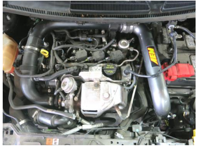
AEM INTAKE INSTALLED
