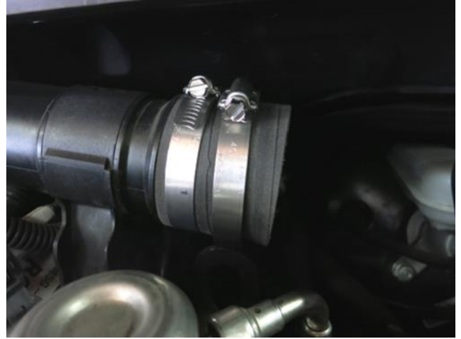
b. Install the small end of the provided coupler onto the intake duct and secure using the provided hose clamps. Leave the right-hand side hose clamp loose at this time.
