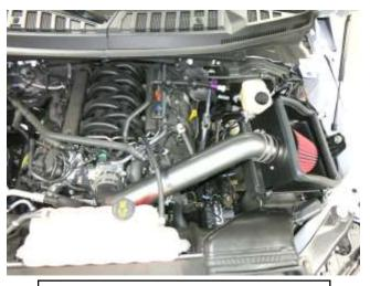
p. Finished installation of AEM Intake System.
