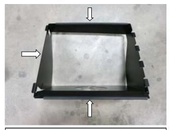
a. Cut two 9.5" lengths from small edge trim and install on bottom of heat shield on opposite ends, as shown. Install remaining length on the third edge as shown.
