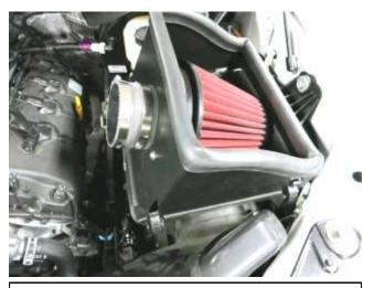
f. Install included straight hose coupler onto filter adapter and secure with provided hose clamp.
