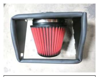
d. Install and secure air filter to air filter adapter using the provided large hose clamp.
