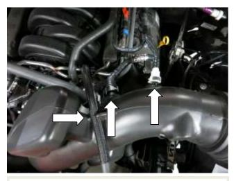
a. Disconnect EVAP vent and crack case vent connectors from factory intake. Pop coolant hose out of notch.
