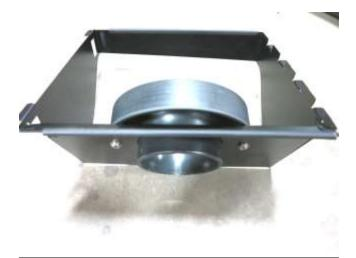
b. Install air filter adapter onto heat shield with provided hardware as shown.
