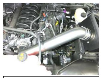
h. Install intake tube at throttle body first, then at air filter. Adjust tube position in couplers for best fit, then secure by tightening hose clamps. Secure heat shield using factory clips at this time.
