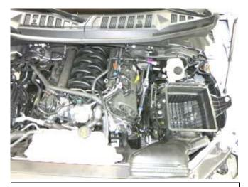
c. Remove intake tube by lifting top half of air box and moving the whole assembly out, from left to right. Remove factory panel air filter. **Retain all stock components.**
