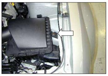
d. Remove the bolt securing the stock air box to the vehicle. Lift up on the stock air box until it is free from the vehicle.
