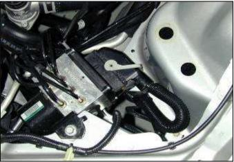
f. Remove the ABS wire harness from the ABS control unit. This is done by pushing in on the locking button and rotating the latch mechanism toward the engine.
