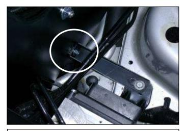
f. Install the lower heat shield mount by using the previously removed lower ABS mount bolt. Use the supplied M6 bolt, nut, and washer to secure the lower mount to the heat shield.
