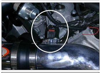
s. Plug in the MAF sensor on the pipe, the throttle position sensor and the throttle plate control motor on the throttle body. Zip tie TPC motor harness to MAF sensor harness.
