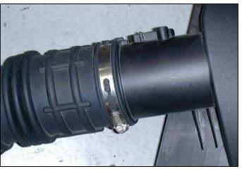
j. Separate the stock intake tube from the air box by loosening the hose clamp securing them. Look inside of the air intake tube to see if there is a carbon trap present and if so procede to next step. Otherwise procede to step 2l.
