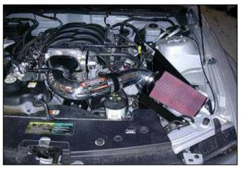
AEM® intake system installed
