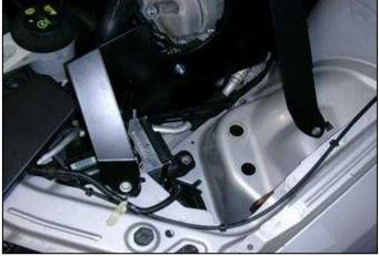
e. Install the heat shield into the engine compartment by carefully sliding it under the AC lines and aligning the two mounting arms with the holes in the fender and upper ABS mount. Secure using the previously removed bolt for the ABS housing and one supplied M6 bolt.
