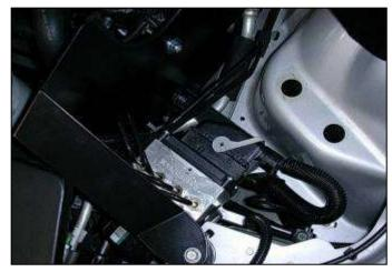
g. Plug the ABS wiring harness back into the ABS control module.
