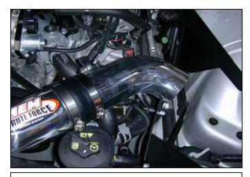
p. Install the lower intake pipe by sliding it into the previously installed coupler. Align the bracket with the rubber mount on the heat shield.
