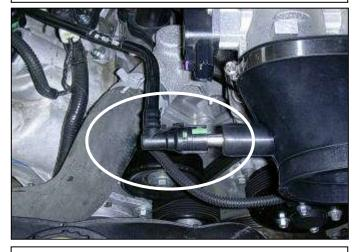
k. Attach the stock plastic breather hose by pushing it over the aluminum nipple until it snaps into place.
