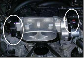
h. Unplug the throttle plate control motor and the throttle position sensor as shown.
