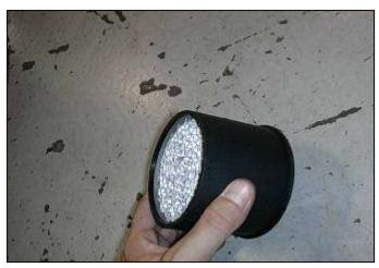
m. Vehicles not equipped with the carbon trap proceed to step 3o. Vehicles equipped with a carbon trap: Install the carbon trap into the supplied rubber isolator. The carbon trap is non-directional and can be installed in the isolator freely.
