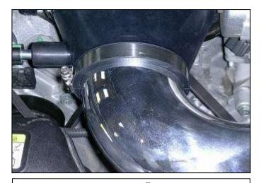
I. Check the inside of the AEM® upper intake pipe to ensure it is clear of any debris. Install the pipe with the bend side into to the previously installed coupler. Secure using a # 56 hose clamp as shown.
