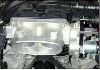
c. Install the throttle body spacer onto the two studs on the intake manifold with the two o-rings facing outward. Install the throttle body using the two previously removed nuts and bolts. Tighten to 84 inch pounds (7.0 ft-lbs).
