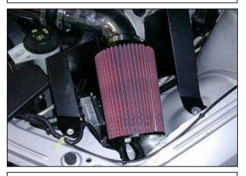
r. Install the AEM<sup>®</sup> air filter onto the end of the inlet tube. Push the air filter over the inlet pipe until the stop in the air filter is reached. Install one hose clamp to secure the air filter onto the inlet pipe.
