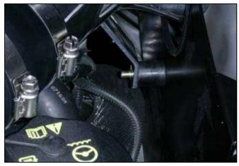
q. Install the M8 washer and nylok nut onto the rubber mount. Leave slightly loose for adjustment.
