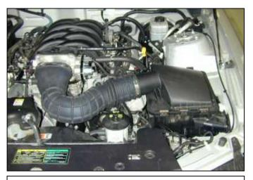
a. Factory air box system installed.
