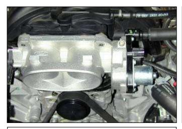
i. Remove the two upper bolts and two lower nuts securing the throttle body to the intake manifold. Set the throttle body aside.
