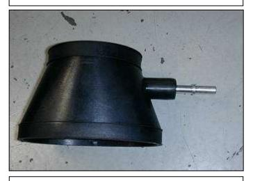
i. Install the aluminum nipple into the EPDM throttle body adapter coupler. This is done by pushing the nipple into the bung from inside the coupler. Next, pull the nipple through until it locks into place.
