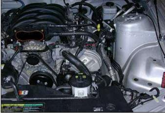
I. Factory air box system removed.
