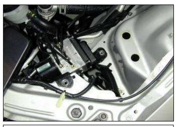
g. Move the harness out of the way and remove the upper and lower bolts securing the ABS unit to the chassis as shown. Set these bolts aside for now as they will be used during installation.
