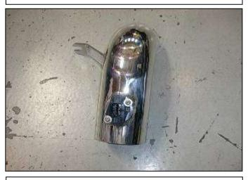
h. Check to be sure that the AEM® intake pipe is clear from debris. Install the MAF sensor using the original mounting screws. Use caution to avoid damaging the o-ring.
