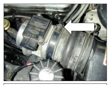
e. Loosen hose clamp and remove MAF sensor. Be careful not to damage sensor or screen.
