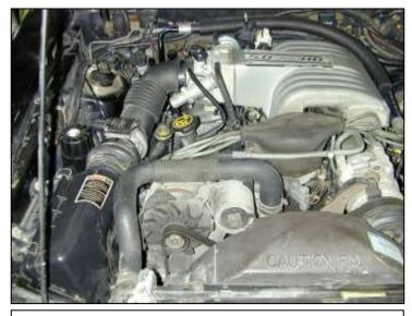
Factory air box system installed
