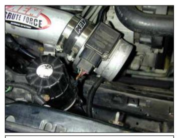
h. Reattach the MAF sensor wire harness connector.
