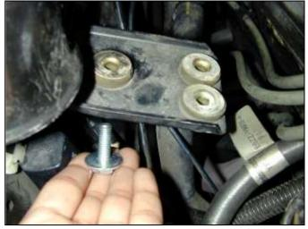
c. Insert M8 bolt into the provided washer.
