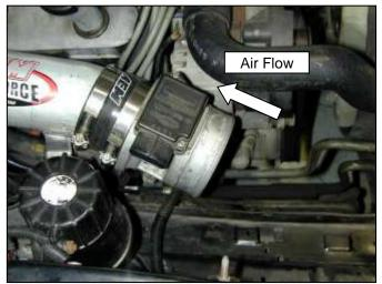
g. Attach the coupler to the inlet pipe and secure with hose clamps. Insert the MAF sensor. **NOTE: Make note of the MAF sensor's air flow direction.**
