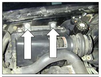
f. Loosen and remove the remaining two nuts on the air box. Remove the air box.
