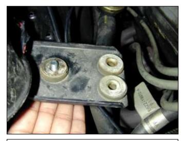
d. Insert the bolt and washer into the hole in the MAF sensor bracket.
