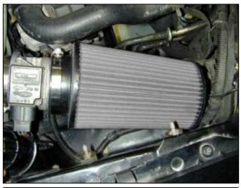
i. Attach the air filter element to the MAF sensor and secure. Check for clearance.
