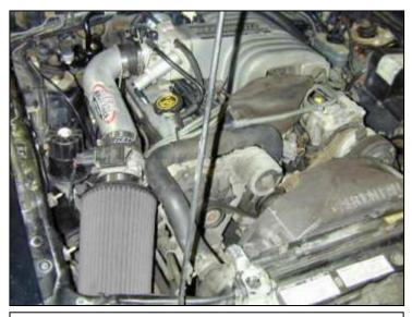
AEM<sup>®</sup> intake system installed
