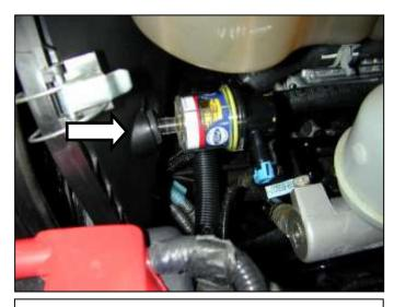
f. Pull the air filter status meter from the grommet.
