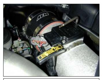
h. **Vehicle with a MAF Sensor:** Install the sensor into the intake pipe using the two factory bolts removed during step 2i. Proceed to step 3k.).
