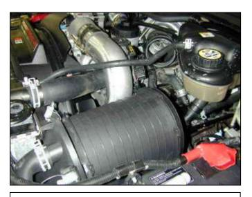
g. Remove the rear section of the intake system.
