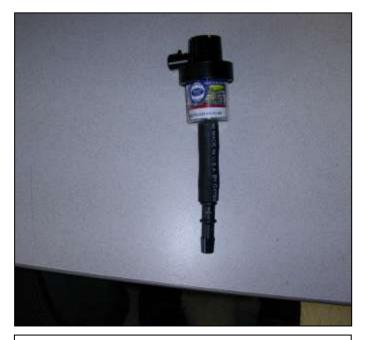
a. If the air filter status meter wire is in tension, add the supplied hose and plastic connector as shown.
