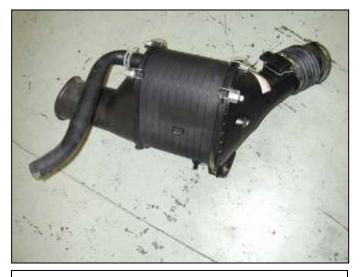
h. Remove the remaining stock air box system.
