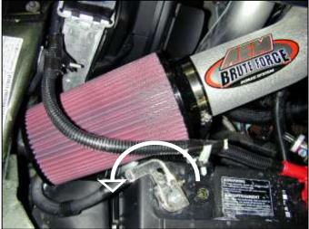
g. Install the air filter onto the end of the pipe. If the negative lead touches the air filter, rotate the terminal, as shown.
