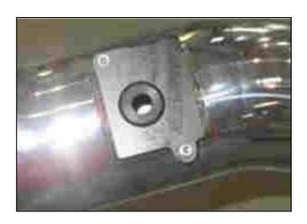
i. On vehicles equipped with an IAT sensor, install the provided adapter plate onto the intake pipe using the two supplied bots. Install the supplied grommet into the plate. Install the IAT sensor into the grommet on the adapter plate and proceed to step 3j.).
