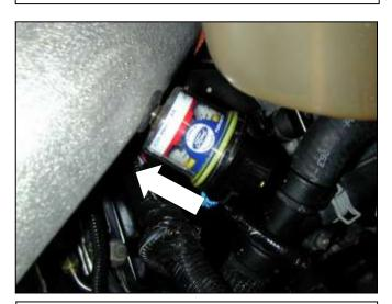
j. Install the air filter status meter into the rubber grommet on the rear of the pipe.
