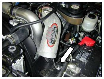
f. Place the inlet pipe in engine bay as shown. Confirm that the mounting tab is under the fender washer.
