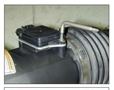
i. Use the supplied torx key to remove the MAF sensor. Save screws for later use.
