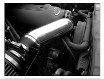
m. Ensure the radiator hose clears the underside of the inlet pipe.
