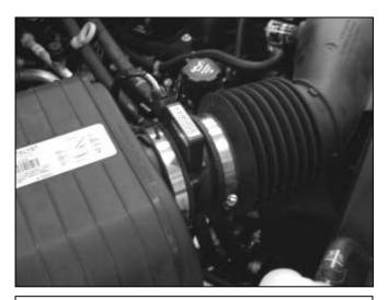
c. Loosen the hose clamp connecting the MAF sensor to the air box.
