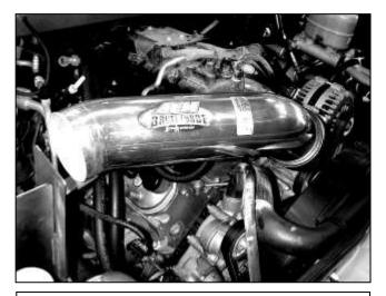
h. Insert the inlet pipe into the 90-degree coupler. Secure with provided hose clamps.
