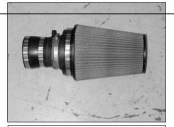
k. Attach the MAF sensor assembly and coupler to the air filter-adapter assembly.
