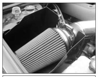
I. Attach the air filter assembly to the intake pipe and secure. Plug in MAF sensor.
