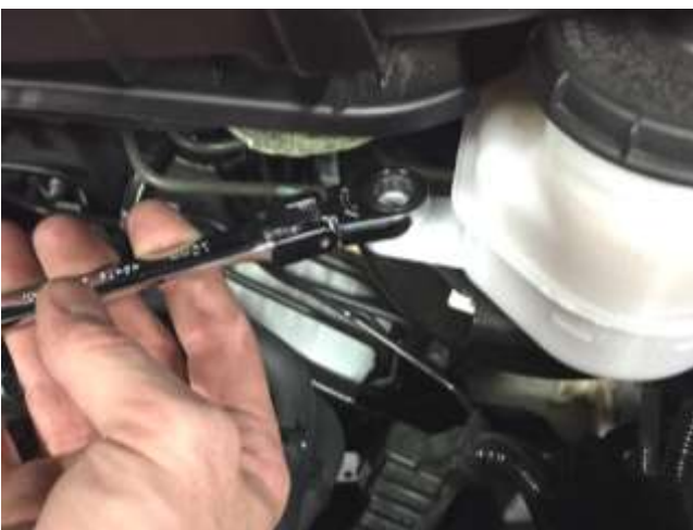
i. Remove the bolt securing the brake reservoir and set aside. It will be reused in step 3j.
