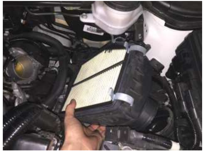
h. Lift and pull the rear air box mount free of its rubber mount and remove the lower air box from the vehicle.
