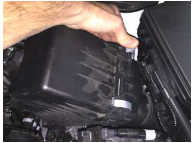
f. Unlatch the two factory air box clips.
