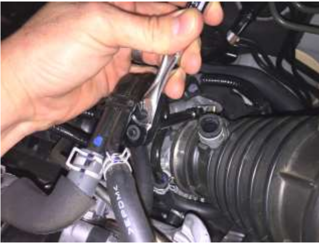
e. Use a Philips screwdriver or a 5.5mm socket to loosen the factory hose clamp on the factory coupler.
