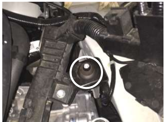
j. Remove the rear air box rubber mount by prying it off of its post . Using soapy water as a lubricant may help. Set this part aside to be reused in step 3a.
