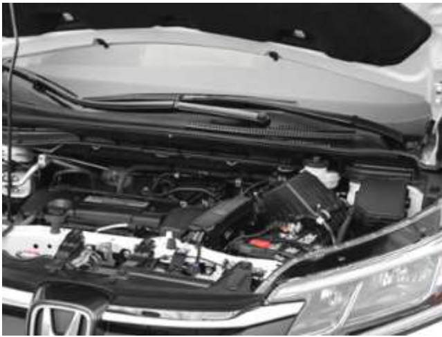
STOCK AIR BOX INSTALLED
