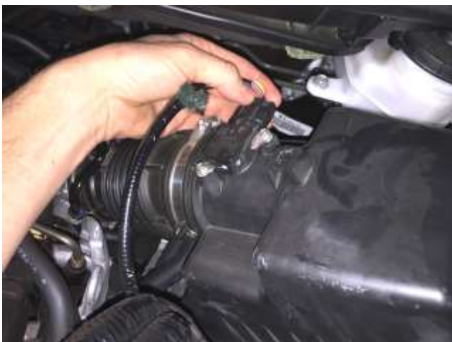
c. Disconnect the mass airflow sensor (MAS) wiring harness and disconnect the wiring retainer clip from the air box. Remove the sensor from the air box and set aside along with its screws to be reused in step 3f.
