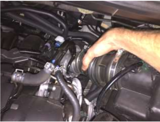
g. Pull the factory coupler off of the throttle body and lift the upper air box assembly out of the vehicle.
