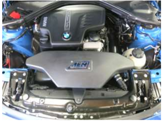
AEM INTAKE INSTALLED
