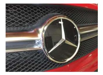
g. To open up maximum airflow to intake, the secondary air inlet must be uncovered. Twist the Mercedes emblem on the grill counterclockwise and pull to remove it. If your car is equipped with Distronic radar-assisted parking and cruise control features, this emblem (shown at right above) will not be removable by twisting in this fashion. The grill will need to be removed to allow removal of the cover as detailed in step 3h below.
