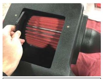
c. Load the filter through the opening in the bottom of the airbox and pass the retainer ring over the filter with the smooth side facing the filter opening.
