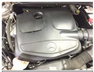
a. Remove engine cover by lifting up at all for corners.
