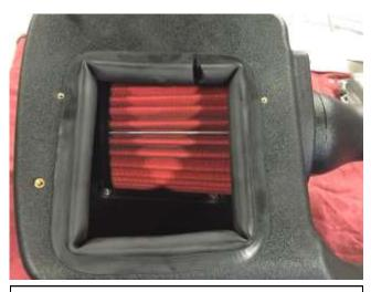
e. Trim 40mm of the remaining edge trim to be used in the next step and install the remainder on the bottom of the airbox as shown.
