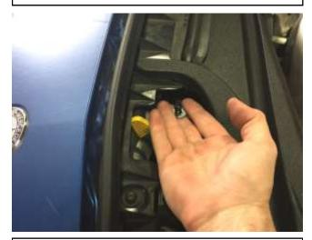
j. Optionally, if the support "finger" on the airbox is not sitting flush with it's mating surface, the included tree clip and washer can be pushed in to the bottom of the "finger" to hold it flush.
