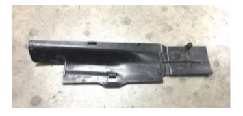
i. The inlet cover may now be removed through the emblem hole. It will look like the piece above. Replace the emblem at this time. Installation is reverse of removal.
