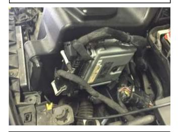
i. With the assembly carefully positioned as shown in the vehicle, use the included M4 bolts and the stand-off assembly to fasten the ECU to the bottom of the airbox. Then, maneuver the entire assembly into position.
