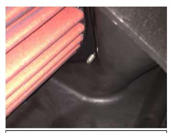
d. Tighten all three mounting screws with uniform torque until about 12mm of the fastener protrudes through the retainer ring.
