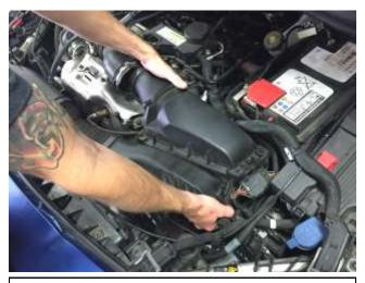
f. Lifting as shown above, remove the factory airbox assembly from the vehicle.
