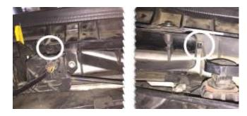
h. Release the inlet cover by squeezing and pushing the cover retainer tabs located on either side of the second-ary inlet.
