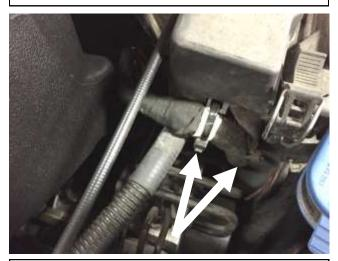
g. Cut the zip ties shown above to free the ECU harness. Take care to not cut the wiring.
