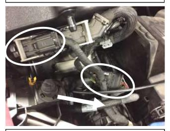
h. Disconnect the two wiring harnesses circled above and pass them under the conduit indicated by the arrow above. Reconnect them both before proceeding.
