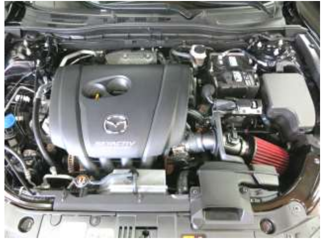
p. Finished installation of AEM Intake System.
