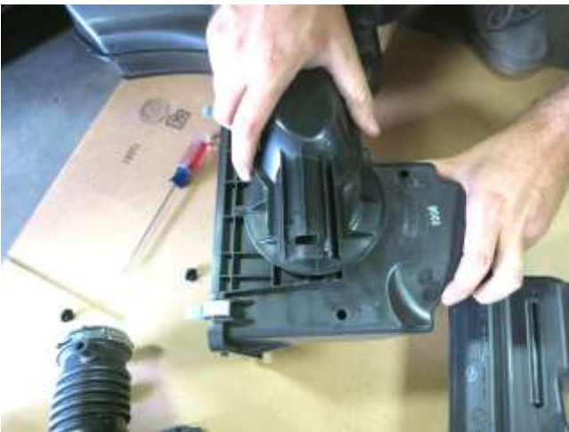
c. Rotate the cold air scoop until it will separate from the lower air box. Note: There are 2 different style scoops used on the vehicle. Both are compatible with this intake system.
