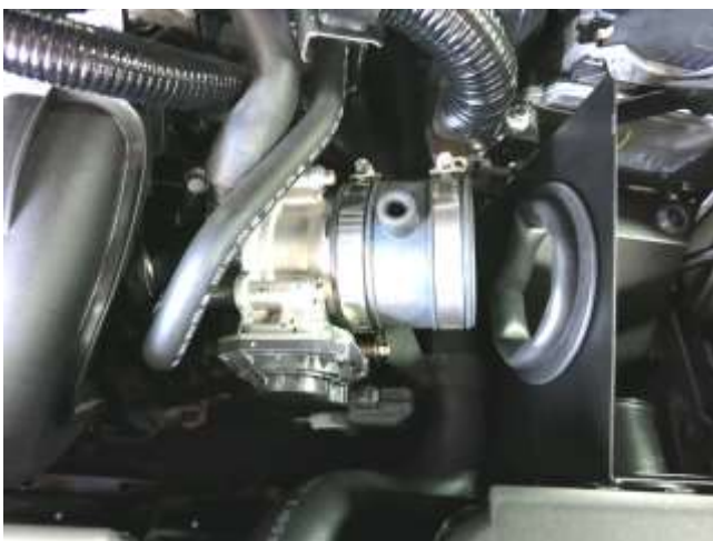
i. Install provided coupler with hose clamps provided onto throttle body with molded port facing upward. Do not tighten hose clamps at this point.
