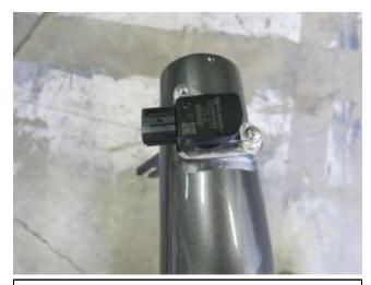
d. Install the MAF sensor that was removed in step 2h. and secure with the provided Allen head bolts.
