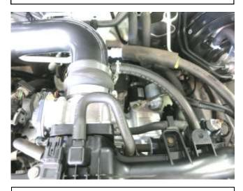
i. Install the new provided vent hose from the AEM intake tube to the engine where step 2g was disconnected.Secure with the factory spring clamps removed in step 2g.
