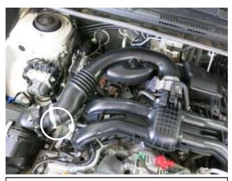
d. Loosen the hose clamp at the air box and remove the stock intake tube from the vehicle.
