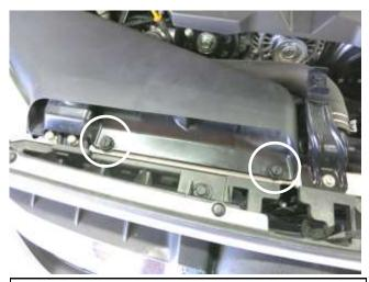
a. Remove the scoop and the two clips from the vehicle.The scoop will not be reinstalled but do not discard.
