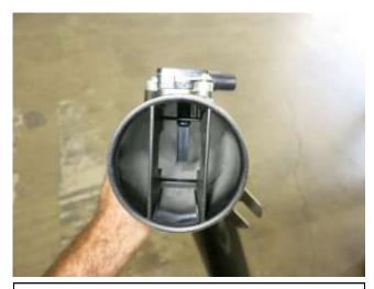
e. Install the MAF insert into the end of the tube and align it as shown. Note: Use a few drips of super glue on the insert's lip to hold it in place in the tube.
