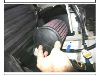
g. Install the AEM filter onto the AEM intake tube from under the vehicle and secure with the provide hose clamp.
