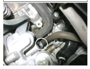
g. Follow the vent line from step 2c to the engine, and release the pressure on the spring clamp, and remove the vent line from the vehicle. Note: The spring clamps with be reused in step 3i.
