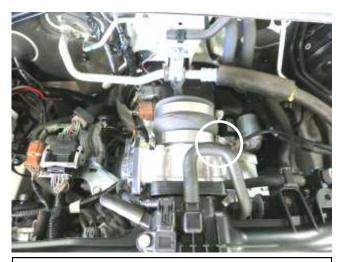
c. Install the provided hose and hose clamps onto the throttle body. Tighten the hose clamp closest to the throttle body now.
