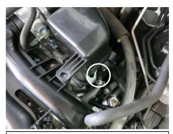
c. Release the pressure on the spring clamp and remove the vent hose underneath the resonator.
