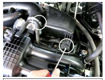
b. Remove the clip securing the stock intake resonator to the engine. Then loosen the hose clamp at the throttle body.
