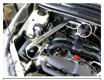
f. Install the AEM intake tube into the vehicle aligning it with the coupler and the hole in the heat shield. Using the provided hardware, secure the bracket to the heat shield. Tighten the hose clamp at this time.
