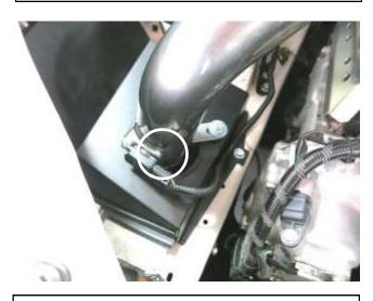
j. Plug the mass air sensor connector back into the mass air sensor.
