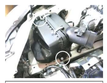
f. Remove the two nuts on the inner fender as well as the bolt on the lower air box. Then remove the air box from the vehicle. The nuts will be reused in step 3b. Note: Do not discard any of your stock equipment.
