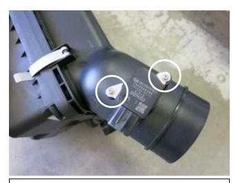
h. Remove the two screws securing the mass air sensor to the stock upper air box lid. Note: The screws will not be reused but the sensor will.
