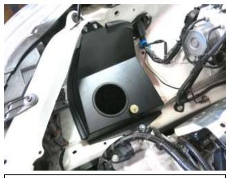
b. Install the AEM heat shield in the vehicle
