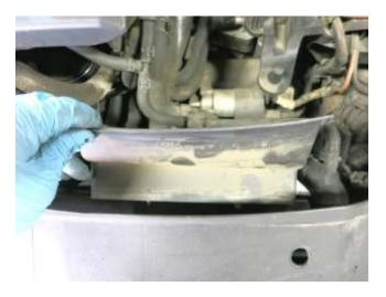
h. Remove the two screws securing the fresh air inlet to the core support and remove it from the vehicle.
