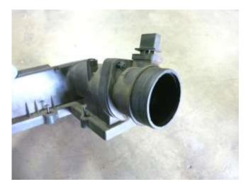
c. Remove the MAF sensor from the factory air box. The MAF sensor is secured with 2 Philips screws.
