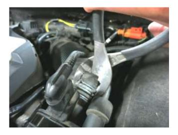
e. Squeeze the spring clamp on the factory air inlet tube with a pair of pliers and release the MAF sensor from the tube.
