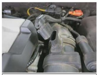
a. Disengage the MAF sensor electrical connector from the MAF sensor.
