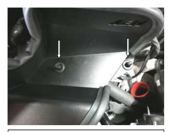
e. Install the heat shield assembly into the vehicle by fitting the grommets over the posts on the air box tray.Fully seat grommets on post. Fitment will be tight.
