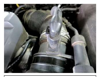
j. Connect the MAF sensor electrical connector to the MAF sensor.
