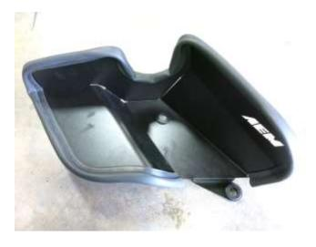
b. Install the supplied rubber edge trim around the heat shield as shown.
