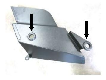
a. Install the supplied rubber grommets into the 2 holes on the heat shield.
