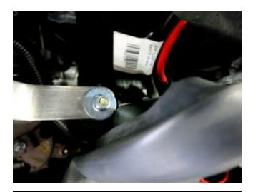
h. Install the supplied M6 nut and washer over the rubber mounted stud but do not fully tighten.
