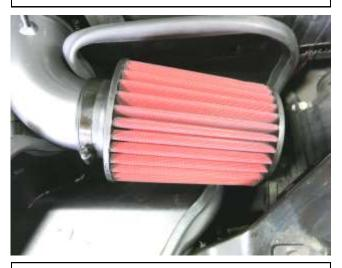
i. Install the AEM air filter onto the intake tube and tighten the hose clamp slightly.
