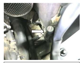
f. Install the supplied rubber mounted stud over the heat shield tab into the threaded boss on the air box tray.
