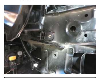
a. Remove the bolt securing the above bracket and replace it with the included rubber mount. Loosely reinstall the bolt with the included washer.
