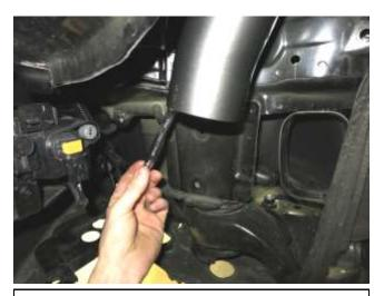
e. Tighten the bolt at the bracket end of the tube with an end wrench.
