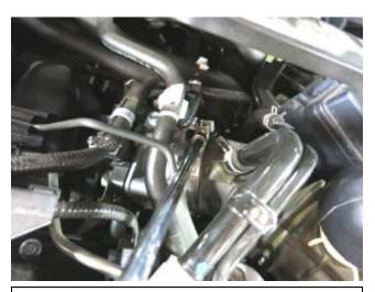
b. Use a cross screw driver or 5.5mm socket to loosen the hose clamp securing the factory intake system to the throttle body. Also remove PCV line from intake boot.
