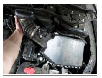
d. Pull the factory intake duct off the throttle body and lift it out along with the airbox.
