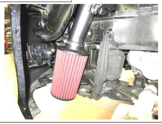
f. Connect the MAF sensor and install the air filter. Install the PCV tube into the adapter at the other end of the tube and seat fully. Reinstall the fender liner and check for clearance at the end of the filter and around the upper edge. If the filter displaces the fender liner, loosen the clamps and bolt, adjust and re-tighten. Reinstall the wheel, taking care to properly torque the wheel to factory specifications.
