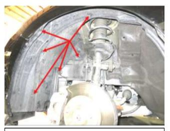
f. Using a flat screw driver, disconnect the nine trim panel clips shown above. Disconnect by inserting screwdriv-
