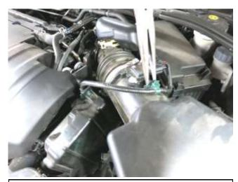
a. Release the green clips retaining the MAF sensor wiring harness and disconnect it from the sensor.
