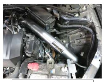
h. Finished installation of AEM Intake System.
