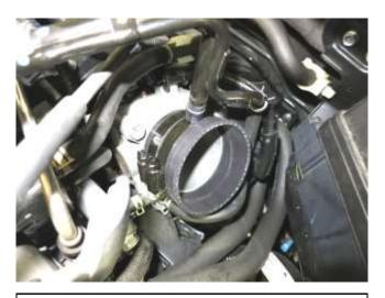
b. Install the included coupler and black hose clamps as shown on the throttle body.
