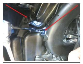
i. First remove the bolt shown above on the left, allowing you to lower the resonator. Using a short 10mm socket and u-joint on the end of at least 14" of exten-
