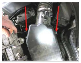
c. Remove the two bolts securing the factory airbox.
