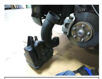
sion, remove the bolt on the right. The resonator can then be pulled out as shown above.
