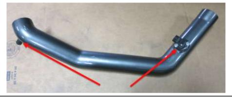
c. Remove the MAF sensor from the factory intake system and install it in your new AEM intake tube with the factory hardware. Also install the rubber tube adapter in the hole at the opposite end of the tube.
