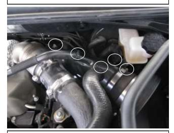
j. Install the AEM intake tube (2-1513C) into the two couplers. Tighten both hose clamps. Install all three of the hoses onto the tube and re-install the spring clamps to secure them that were removed in 2c.
