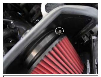
k. Install the AEM filter (21-209DK) and hose clamp (94104) onto the filter adapter and secure the hose clamp.
