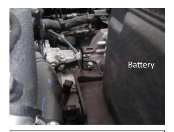
a. Install the supplied bracket (32-3095), bolt (08373), and washer (08275) onto the angled part of the battery tray as shown. **Note:** The 90° bend will be at the top part of the bracket.
