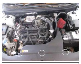
I. Install the stock scoop and plastic screws that were removed in step 2a. Then reinstall the engine cover.
