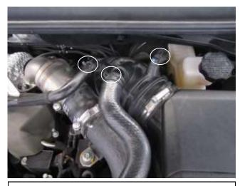
c. Release the 3 spring clamps circled on the stock intake tube and remove the 3 lines attached to the stock intake tube. These will be reattached in step 3j.
