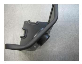
d. Install the adapter (21512-1) with the supplied button heads (07730) and 2 washers (1-3025 & 08275).
