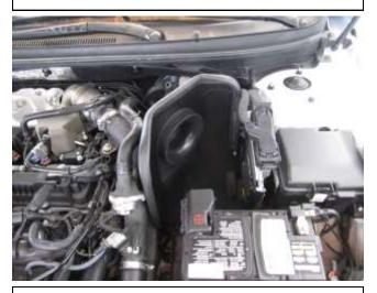
h. Install the completed heat shield into the vehicle aligning the 2 slots in the front to the previously installed mounts. Push down to secure the stand off.
