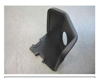
c. Install the edge trim(102487) as shown. Cut the trim to fit all three sections.
