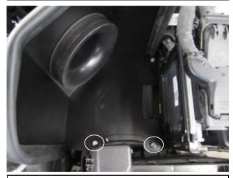
i. Install a washer (08275) and nut (07529) onto the rubber mount, shown on the right. Then install the bolt (08373), 2 washers(08275), and nut (07529) to secure the heat shield to the bracket. **Ref.** Exploded View
