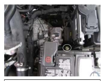
b. Install the rubber mount (1228599) into the battery tray location shown.
