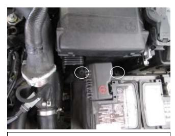
b. Remove the 2 bolts securing the stock air box to the vehicle.
