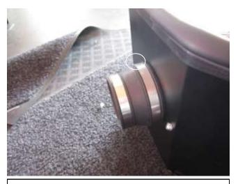
f. Install the hose adapter (5-1046) onto the filter adapter with hose clamps (9448 & 9456). Tighten the hose clamp closest to the heat shield at this time.
