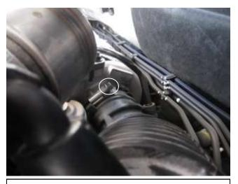
d. Loosen the hose clamp at the throttle body and remove the stock air box/intake tube from the vehicle.
