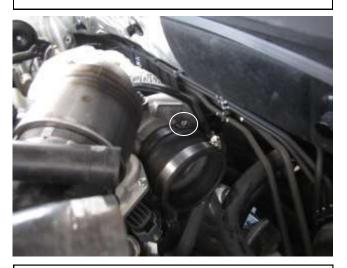
g. Install the hump hose (5-574) onto the turbo with the supplied hose clamps (9440 & 9448). Tighten the hose clamp closest to the turbo at this time.
