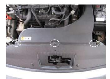
a. Remove the engine cover by pulling it up and out of the vehicle. Then, remove the 3 plastic screws circled and pull the stock scoop out of the vehicle.
