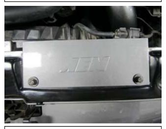
I. Install the heat shield onto the front radiator support using the provided bolts (1-2038)
