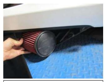
i. Place the AEM filter up into the wheel well above the splash guard as shown.
