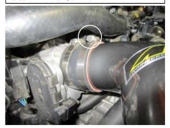
e. Install the tube into the throttle body coupler and tighten the hose clamp. **Note:** Make sure there is clearance between tube and coolant lines.
