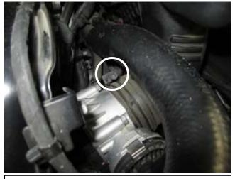
b. Loosen the hose clamp at the throttle body.
