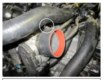
b. Install the coupler and hose clamp (9448) onto the throttle body and tighten.
