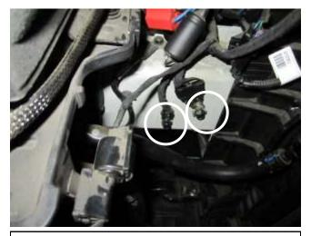
f. Remove the bolts circled on the drivers side chassis.You will only be reusing the bolt on the right in step 3a.
