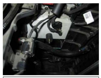
a. Install the rubber mounted stud into the bolt hole that was removed in step 2f. Combine both ground cables together and tighten the bolt back up.
