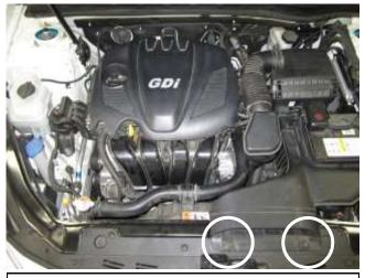
a. Remove the engine cover by pulling up and out of the vehicle. Remove the two bolts holding the air scoop to the vehicle and remove the scoop.
