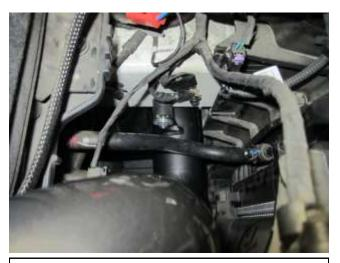
d. Slide the tube into the wheel well, align the bracket with the rubber mounted stud. Install/tighten the washer and nut to secure the tube. **Note:** The tube will go between the two flex lines that run to the radiator.
