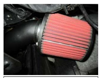
j. Slide the AEM filter onto the tube and tighten the hose clamp (9452). **Note:** Rotate the offset-base filter as necessary to gain best clearance.
