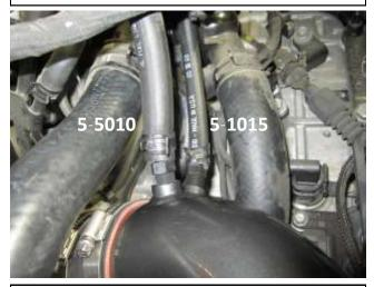
f. Install the hose (5-5010) and (5-1015) onto the fittings and secure with the pressure clamps that were removed in step 2d.
