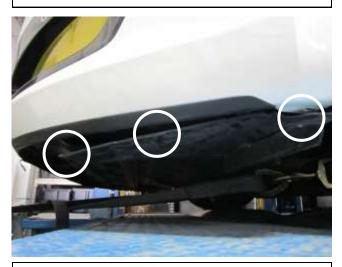
k. Install the 3 screws that were removed in step 3h.
