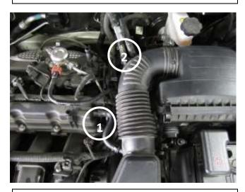
d. Loosen the #1 pressure clamp and remove the vent tube. On vehicles equipped with an EVAP vent line, disconnect the #2 pressure clamp and remove the EVAP hose from the "T" fitting. All four of the pressure clamps will be re-used in 3f & 3g.
