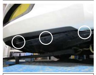
h. Remove the 3 screws holding the drivers side splash guard and lower the guard.
