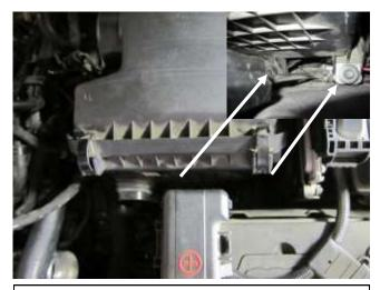
e. Remove the stock intake tube, then remove the two bolts securing the stock air box. **Note:** Do not discard any of your stock equipment.
