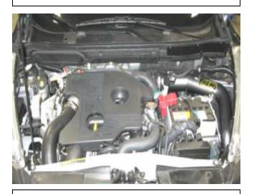
j. Finished installation of AEM Intake System.
