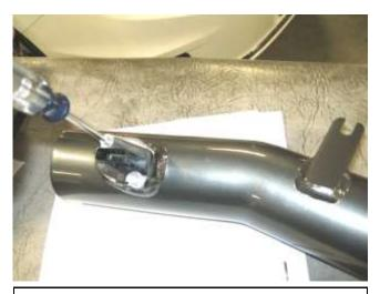
a. Install the MAF sensor onto the intake tube and secure with the two M4 screws that were removed in step2j.
