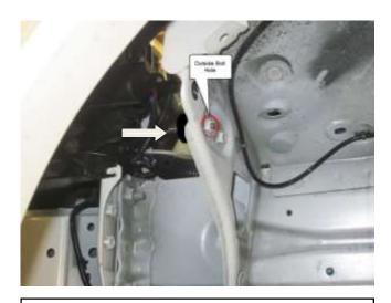
c. Install the second rubber mounted stud into the "outside" bolt hole in the fender well brace, make sure to capture the harness bracket, and tighten.
