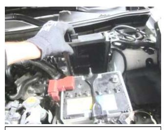
f. Remove the stock air box from the vehicle. **Note:** Remove the rubber bushings under the air box and keep with air box as they will not be utilized.
