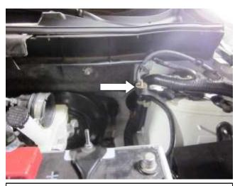
b. Install one of the provided rubber mounted stud in the bracket where you removed the M6 bolt in step "C" and tighten.
