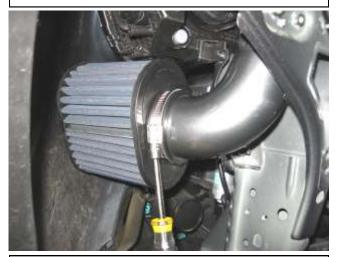
g. Install the AEM air filter onto the intake tube and tighten the provided hose clamp. On some trim models, the air filter may need to be rotated to fit properly.
