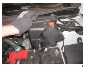
d. Remove the upper half of the air box with the filter still intact band lift both out of the engine compartment.
