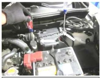
c. Loosen the hose clamp, remove the M6 bolt, and disconnect the two latches securing the air box lid to the base.
