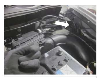
b. Lift up on the air box tab and pull out the locating pin on the stock air intake tube.
