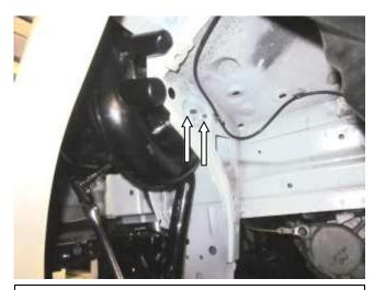
i. Remove the two M6 bolts in the fender well brace that holds resonator and harness bracket in place.
