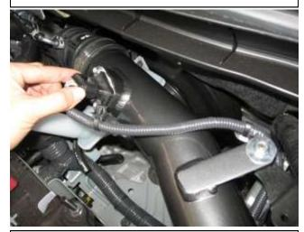
h. Install the MAF sensor connector onto the MAF sensor that was removed in 1a and reinstall fender well liner and wheel in reversed order outlined in step 2h.
