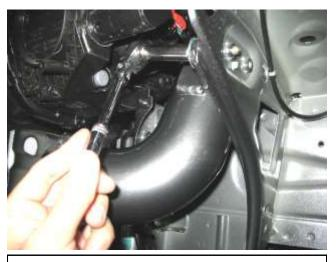
f. Align the lower portion of the AEM intake tube bracket on top of the rubber bushing and tighten the provide M6 nut/washer.
