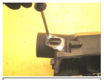
j. Remove the two M4 Screws and pull out the MAF sensor. **Note:** Handle with care. The sensor and screws will be reused in step 3a.
