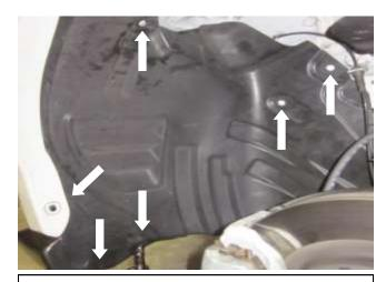
h. Raise vehicle to remove left front wheel. Remove the four locating tabs and the two M6 bolts that hold the wheel well liner in place. Position the liner out of way.
