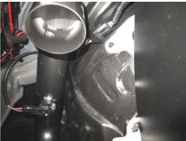
i. Connect the MAF extension harness(8-197-1) to the stock harness, around the tube, and plug into the MAF sensor.
