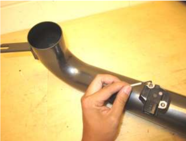
a. Install the mass air flow sensor that was removed in 2h) into the AEM intake tube with the supplied hardware (1-2051) using 4MM Hex Key.
