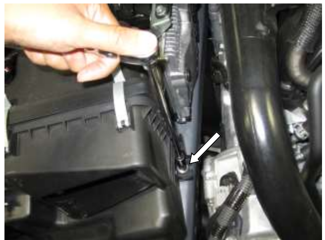
d. Remove the bolt that secures the air box to the engine bay and set aside for late use with AEM heat shield.
