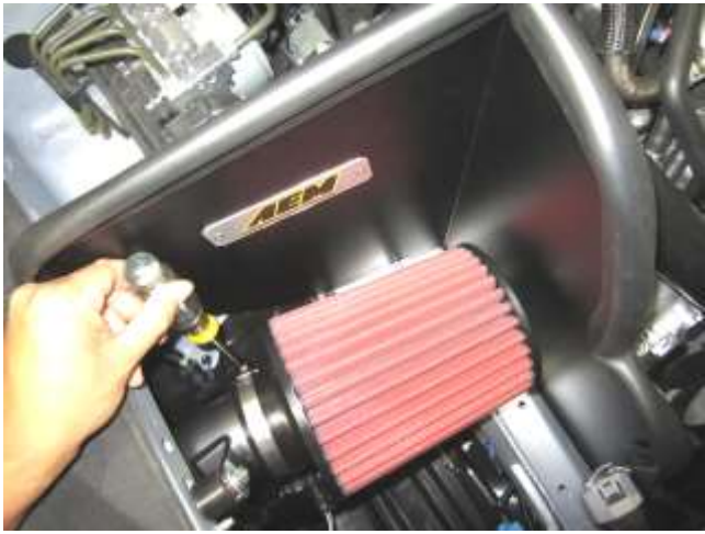
l. Install AEM DryFlow filter(21-2027DK) and secure to intake tube using hose clamp(9448) .
