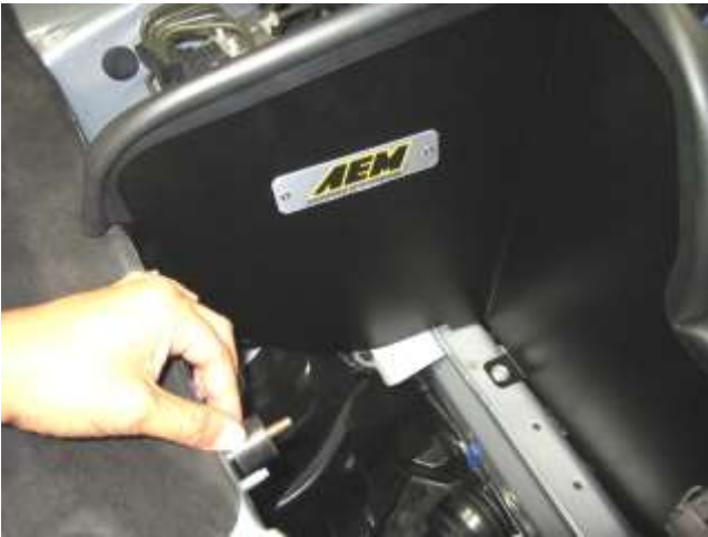
g. Install the provided rubber mount(1228596) as shown .
