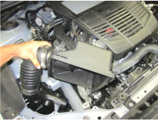
g. Slide the intake tube off the lower bellows coupler and remove tube/box assembly from engine bay.
