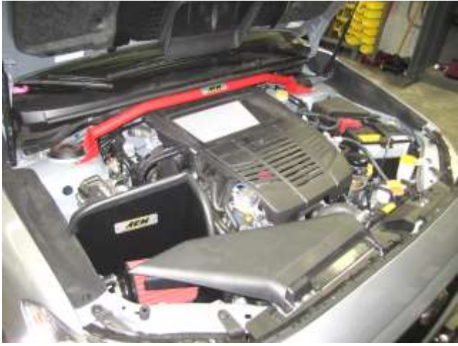
n. AEM intake installed.
