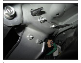
I. Remove the 1 bolt and 2 nuts securing the bumper cover to the driver side fender where the fender liner was removed.
