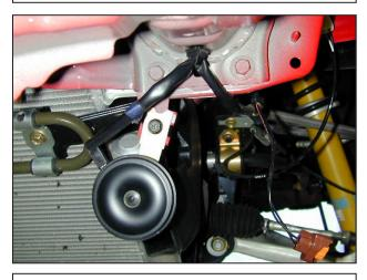
i. Re-install the clip for the horn wiring harness from the horn to the front bumper support. Re-install the clips attaching the IAT sensor and wiring harness to the bumper beam.
