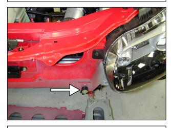
c. Install the supplied M6 isolator mount (F) in the location shown. Secure using the supplied M6 flat washer (G) and M6 nut (H).
