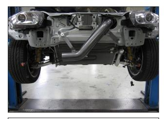
e. Loosely mount the lower intake tube (A) brackets to the isolator mounts as shown using 2 flat washers (G) and 2 M6 nuts (H) turned finger tight.
