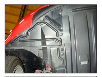
f. Remove the retaining clips and bolts securing the driver side splash shield to the vehicle. Remove the splash shield.
