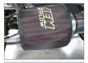
g. Install the AEM® prefilter (L) over your new AEM® Dryflow air filter (B), then mount the filter onto the end of the lower intake pipe using the #52 hose clamp (K) and fully tighten.
