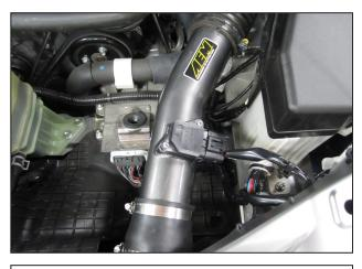
f. Install the lower tube into the reducing coupler on the upper intake pipe and align the tube brackets with the rubber mounts. Once aligned, secure the pipe with the #48 hose clamp (J) and then fully tighten the 2 M6 nuts from Step e. with a wrench.
