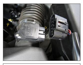
b. Unplug the MAF sensor from the wiring harness.
