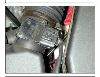
u. Remove the MAF sensor from the stock housing using a screwdriver.
