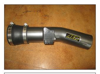
a. Install the MAF sensor into the upper intake tube (D) and secure using the two supplied 8-32 Allen bolts (E). Install the reducing coupler onto the end of the intake pipe and secure with the #44 hose clamp (I). Loosely install the larger #48 hose clamp (J) onto the end of the coupler.
