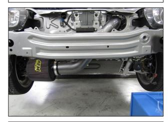
h. Re-install the front bumper assembly using the 8 factory bolts. Ensure the air filter or intake tube does not contact any part of the vehicle.
