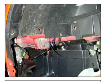
i. Remove the clips and bolts securing the driver side front fender liner and remove the liner. Disconnect the fog light and side marker light from the wiring harness.
