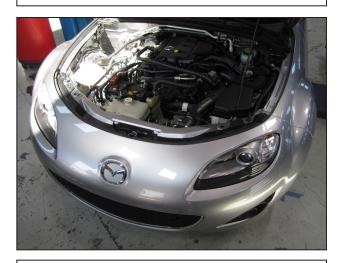
n. Remove the 8 bolts securing the bumper cover to the top of the radiator support.
