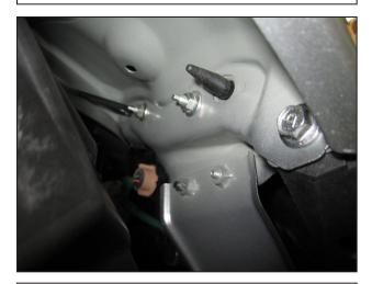
m. Remove the 1 bolt and 2 nuts securing the bumper cover to the passenger side fender where the fender liner was removed.
