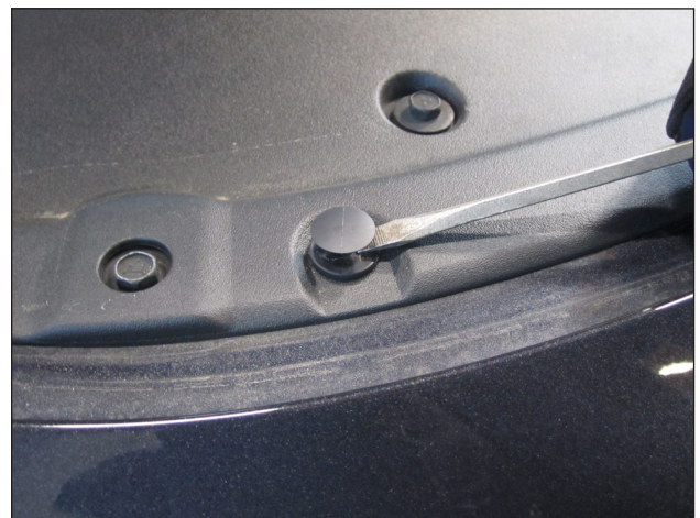
j. To remove the clips, lift the center with a flathead screwdriver to unlock them, then remove the clip.
