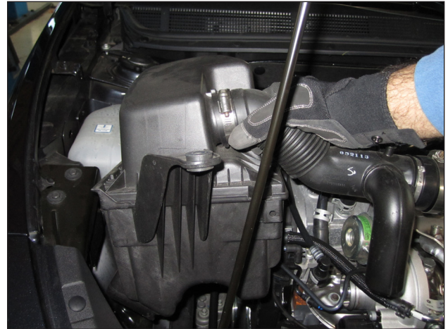
h. Carefully remove the upper intake tube and air box assembly from the engine compartment.
