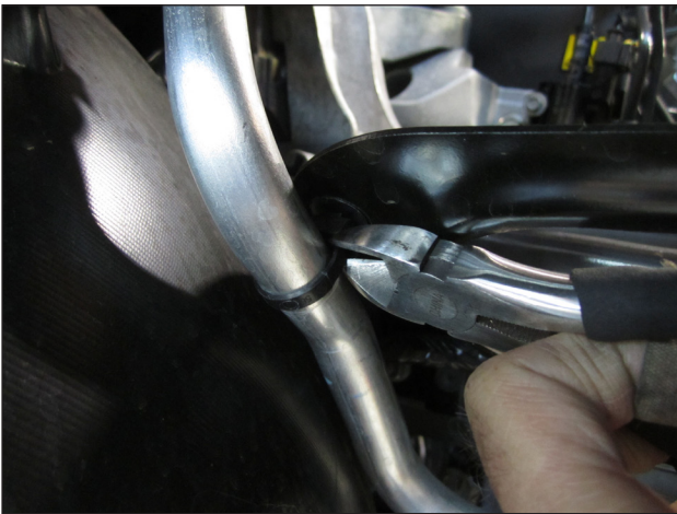
y. Remove or cut the clip holding the heater tube to the intake mounting bracket.
