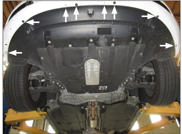
n. Remove the 8 bolts around the lower edge of the front bumper.
