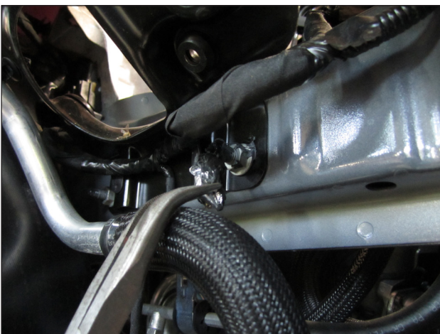
aa. Remove the aluminum insulator shield and putty from the stud to access the right hex nut.
