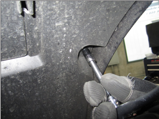
m. Using an 8mm socket remove 10 bolts: 5 along the edge of the right front wheel liner, and 5 along the edge of the left wheel liner.
