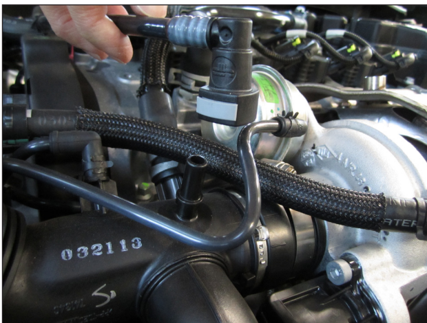
c. Disconnect the quick-release vacuum port at the stock intake tube by squeezing the gray tabs.
