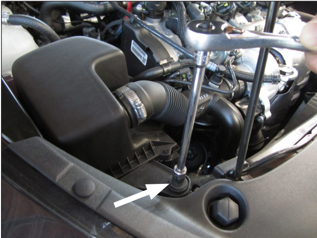
a. Remove the engine cover if equipped. Remove the M6 bolt at the air box mounting flange.
