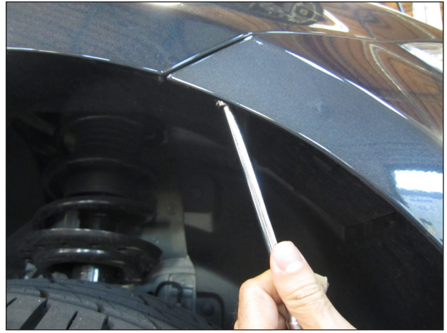
i. Remove the 2 M6 bolts, 1 under each front wheel well at the edge of the front bumper cover.
