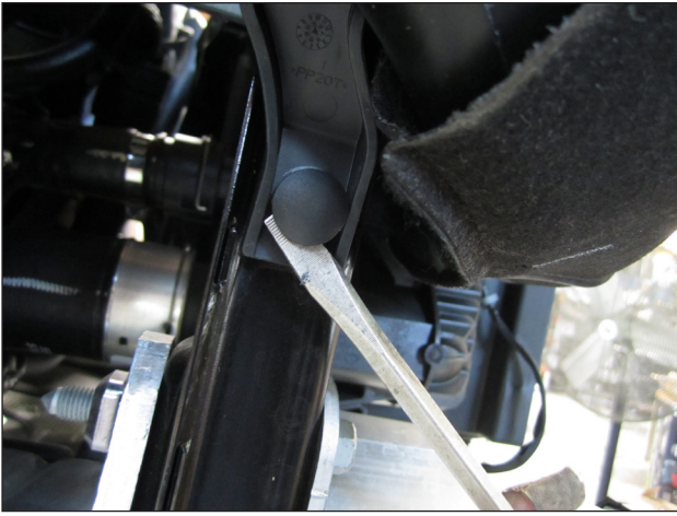
w. Remove the clip holding the lower inlet tube bracket to the outside of the right radiator support.
