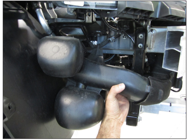
x. Remove the lower inlet tube and resonator assembly from the intake mounting bracket.
