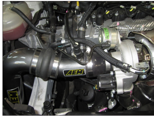
l. Now fully tighten the hose clamp securing the lower intake tube to the hump hose.
