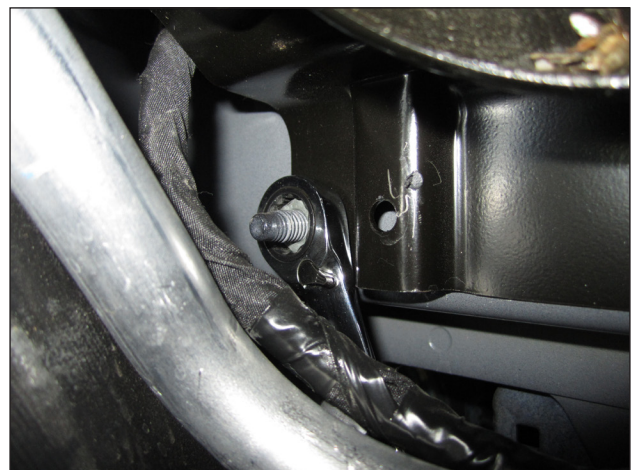
ab. Remove the two hex nuts holding the mounting bracket, then remove the bracket.
