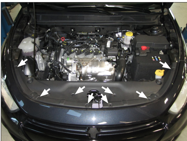
i. Remove the 8 clips holding the vanity cover over the radiator core support.
