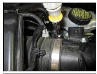
Lossen the hose clamp on inlet tube to the airbox.
