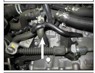
Use the provided zip tie (15) to attach the transmission vent tube to the coolant line as shown.
