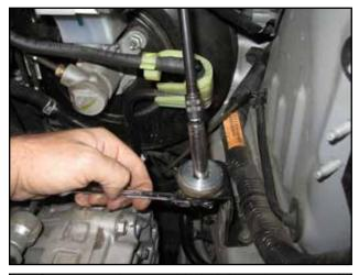
Once properly assembled, tighten the nuts and bolts to secure the adapter assembly.
