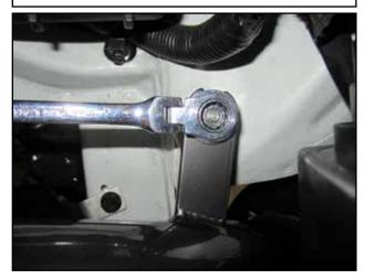
p. Now tighten the M6 (11) nut on the intake tube bracket.
