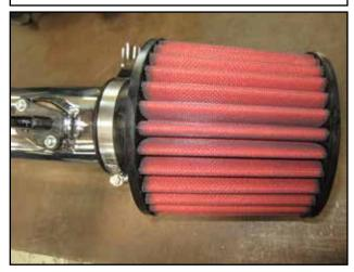
. Mount the AEM air filter (2) onto the intake tube (1) using the (6) hose clamp. Tighten Hose clamp.
