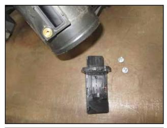
k. Remove MAF sensor from the air box.
