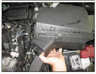
g. Lift up on the bottom of the airbox to disengage but do not remove from the engine bay.
