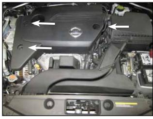
Remove the three Allen head bolts that secure the engine cover in place.
