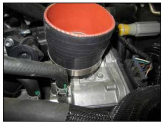
c. Install coupler (3) and hose clamp (5) onto the throttle body and tighen the hose clamp.
