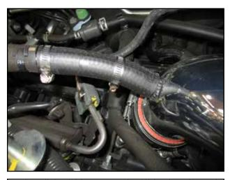
m. Install the (7) hose onto the (1) intake tube and insert the (8) nipple into the OEM vent hose as shown.
