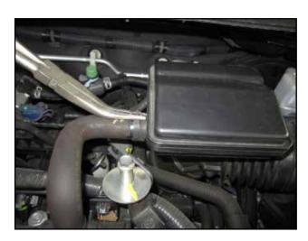
c. Remove the spring clamp securing the PCV hose to the stock intake tube, then remove the hose from the vent.
