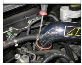
o. Tighten the provided (7) vent hose and (8) hose clamp to the intake tube.
