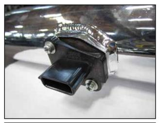
Install the MAF sensor into the intake tube (1) using the OEM screws.
