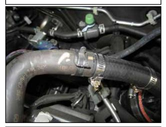
Secure the vent hose on the nipple with the OEM clamp.
