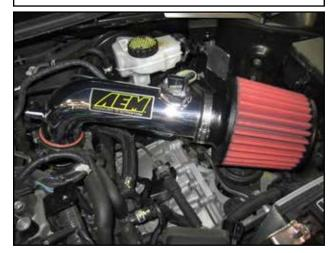
Install the intake pipe (1) into the throttle body coupler and align the bracket in place on rubber mount.
