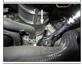
Loosen the hose clamp on inlet tube to the throttle body and remove hose.
