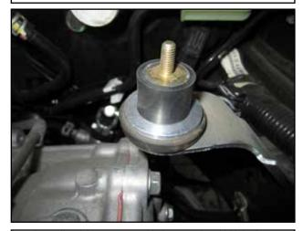
h. Install rubber mount (14) onto the (12) bolt.
