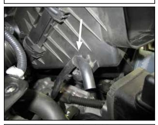
Undo the clip on the airbox holding the transmission vent hose. Undo the transmission vent hose clip from the airbox.
