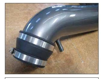
k. At the top end of the upper intake tube, install the reducer coupler, one #56 clamp and one smaller #48 hose clamp. Loosely tighten the hose clamps.
