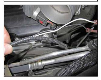
i. Slip the protective convoluted split-loom wire cover over the newly extended IAT wire harness. Trim as needed.
