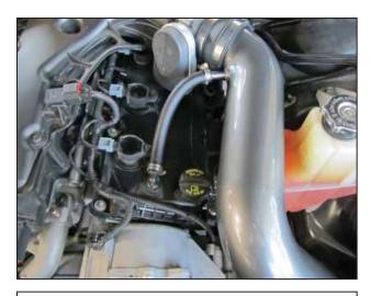
p. Install the supplied  $\frac{1}{2}$ " ID hose between the crank case vent on the head cover and the nipple on the upper intake pipe using the provided small hose clamps. Trim the hose if needed.
