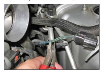
b. Slit open the insulation cover at the end of the IAT connector cable to expose the 2 wires. Cut the wires 1-2 inches [5 cm] below the connector.
