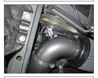
n. From underneath the vehicle, plug the IAT connector onto the IAT sensor in the lower intake tube. Be sure to pull up the red lock tab to secure the connector (if applicable).
