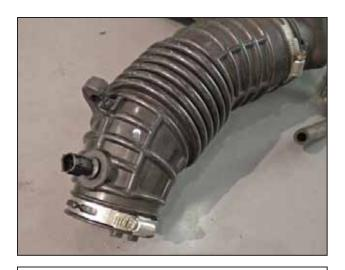
e. Carefully remove the IAT sensor from the OEM rubber inlet hose. Set the sensor aside for future use.
