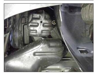
h. Locate and remove the 10mm bolt securing the lower intake resonator to the vehicle. Remove the resonator.
