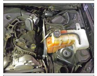
d. Pull the rubber inlet hose off of the throttle body, then lift and remove the OEM air box assembly.
