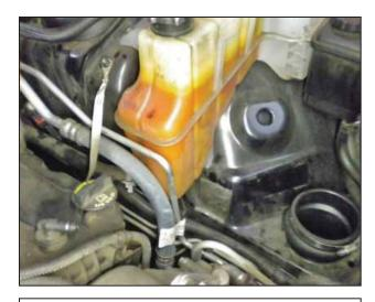
I. Install 1 #56 hose clamp onto the lower elbow hump hose coupler as shown.
