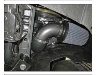
i. Install the lower pipe assembly as shown, using one M8 washer, one M8 nut, and one #56 clamp.
