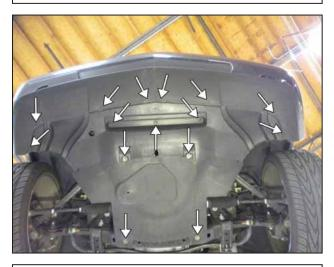
g. From underneath the vehicle, remove the following: 3 clips, 7 screws, and 2 bolts from the front belly pan. Remove the front belly pan.
