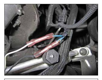
g. Crimp the stripped stock wires into the new Perma-Seal connectors on the black and white wires. Since the color of the stock wires may vary with each vehicle, pay close attention and crimp the other ends of the new black and white wires to the correct color wires on the IAT connector.
