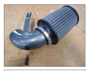
g. Install the grommet into the lower pipe. Attach the air filter with one #56 clamp as shown.
