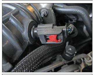
c. Unplug the IAT sensor. To unplug the IAT sensor, slide the red tab back to unlock the latch on the plug, then press in on the latch and pull the plug off of the sensor.
