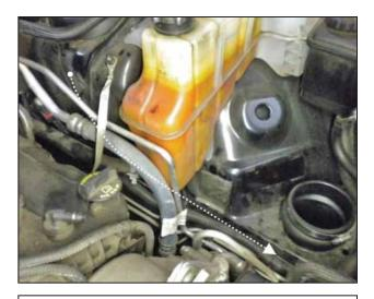
m. Route the new IAT extension harness underneath the existing OEM factory harness as shown. Use the 2 supplied zip ties to secure the extension harness and route the female connector down below to the lower intake tube.
