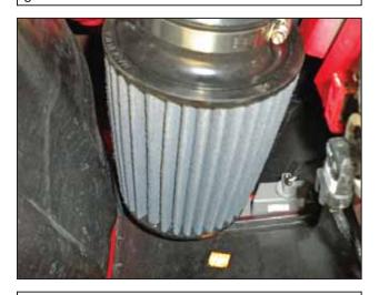
j. Adjust the lower pipe assembly so that there is equal space between the filter, bumper support, fender liner, and marker lamp. When a good fit is achieved, tighten both nuts on the rubber mount and the #56 clamp.
