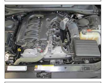
Stock air box system installed
