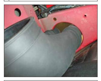
d. From underneath the vehicle, hold the collapsed coupler firmly and insert it through the large hole in the sheet metal.
