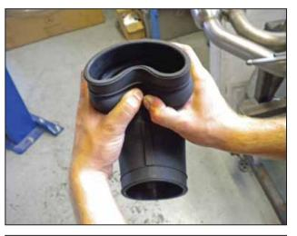
c. Hold the rubber coupler as shown, and squeeze the hump end of the coupler to collapse it into itself.
