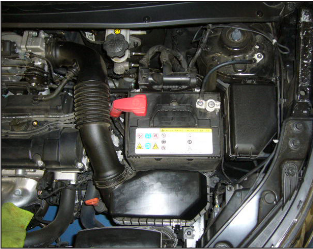
Factory airbox system installed
