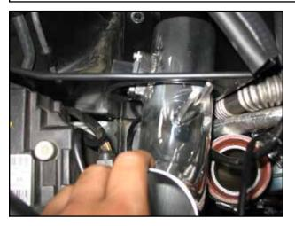
t. Insert the inlet pipe into the heat shield as shown with the bracket facing up and MAF sensor facing toward the passenger side of the car.
