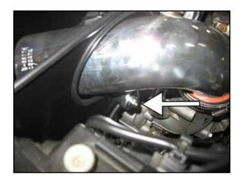
w. Insert the pipe into the coupler and align the bracket with the rubber mount on the heat shield. Secure the bracket with the supplied M6 washer and nut.
