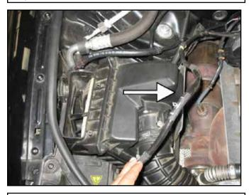
i. Pull the MAF wire harness carefully away from the stock air box.
