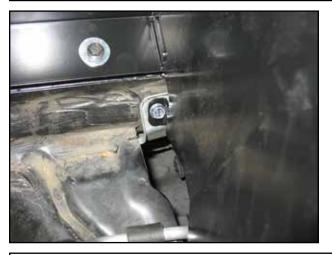
I. Install the supplied M6-1.0X20 bolt through the heatshield and the spacer. Thread it into the hole exposed in step 2q.
