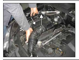
o. Grab the stock air box in the locations shown and move it toward the engine by two inches. Pull the assembly straight out of the engine bay (keep a firm grip and pull hard).
