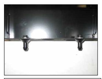
d. Insert the two M6X12 bolts and washers into the two holes on the bottom of the heat shield. Screw the heat shield mounts onto the bolts holding the heat shield mount with your hand. Then tighten the bolts with a 10mm wrench or socket.
