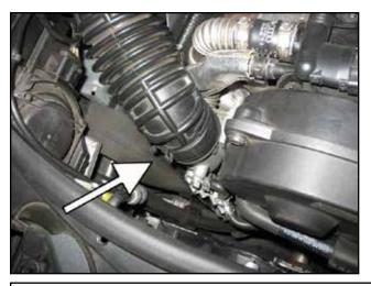
I. This is a good location for the hose clamp to be located once you have moved it away from the rubber inlet tube and turbo inlet joint.
