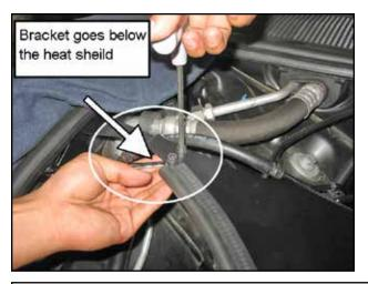
q. Align the M6- 1.0X14 socket bolts with the two holes on the heat shield and bracket. Secure the M6 bolts with the supplied M6 nuts.
