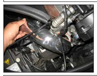
u. Once the sensor has passed through the inlet hole, rotate the pipe 180 degrees clockwise to align it with the coupler on the turbo inlet.
