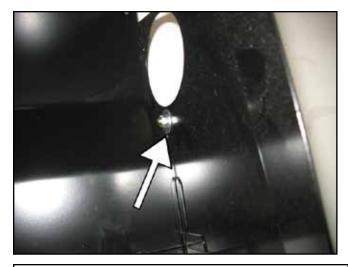
e. Insert the rubber mount into the hole located just below the pipe inlet hole and secure the rubber mount with a washer and an M6 nut.
