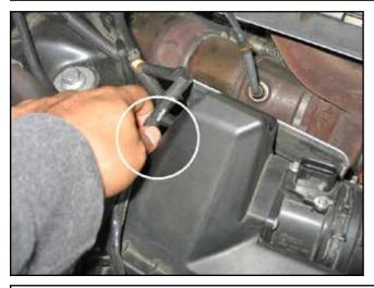
h. The third clip is located on the firewall side of the air box.
