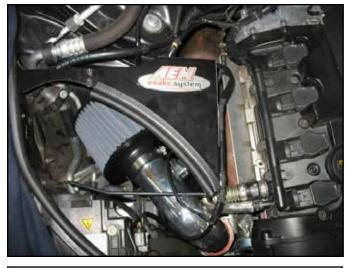
AEM<sup>®</sup> intake system installed
