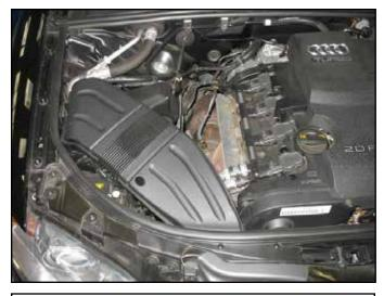
Factory air box system installed
