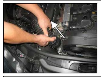
m. Firmly grip the rubber inlet using two hands to pull the rubber inlet away from the turbo inlet.
