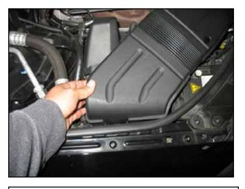
c. Carefully lift the back side of the fresh air duct away from the air box.
