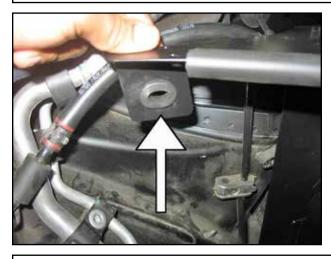
m. Install the 1/2" grommet supplied in kit, into the small oval hole located on the tab on the back of the heat shield.
