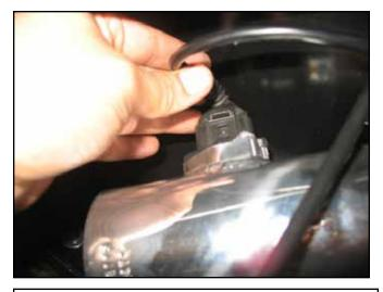
v. Plug the MAF sensor harness into the MAF sensor.
