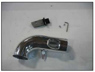
b. Use the stock MAF sensor screws and the supplied tamper-proof torx tool to secure the MAF sensor to the inlet pipe.
