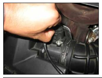
f. Disconnect the mass aiflow (MAF) sensor harness from the MAF sensor.
