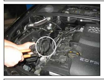
n. Carefully decompress the hose clamp again and remove it from the rubber inlet tube.
