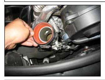
s. Put the transition coupler on the turbo inlet. The #40 hose clamp goes on the turbo inlet side and the #44 hose clamp goes on the inlet pipe side.
