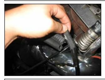
y. Secure the three metal clips located on the MAF harness wire to the heat shield. There are three holes located on the sides near the top.
