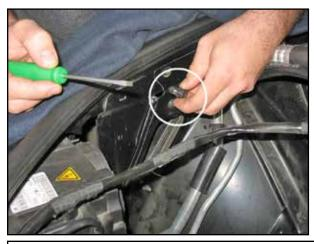
p. Using a small flat screwdriver, remove the plastic receiver off of the plastic rivet removed in step 2j.
