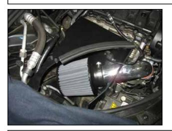
x. Install the Dryflow  ${}^{\rm TM}$  air filter and secure it to the end of the inlet pipe with the #48 hose clamp.
