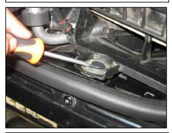
j. Remove the plastic rivet securing the air box to the passenger side fender by using a flat screwdriver to pry it off.
