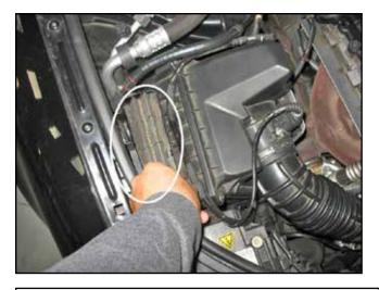
e. Remove the prefilter from the stock air box. This may still be in the fresh air duct.
