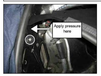
r. Apply pressure with your hand on the bracket toward the passenger side fender and tighten the machine screw with a phillips head screwdriver until it feels secure.
