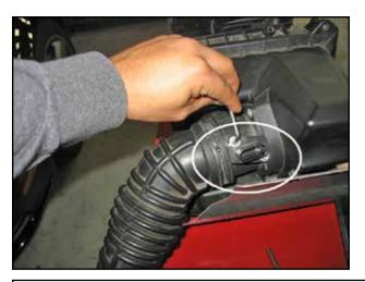
r. Carefully remove the MAF sensor from the stock housing using the supplied tamper-proof torx tool.
