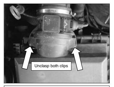
c. There are 2 clips holding the air box to the MAF sensor. Unclasp the metal clips holding the MAF sensor to the air box. Remove the stock air box assembly.
