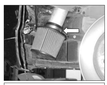
h. Attach the air filter. Secure with provided hose clamp.
