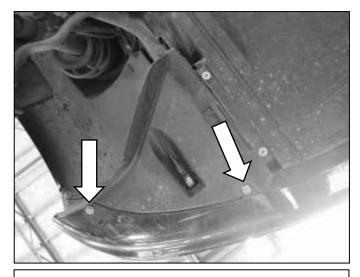
g. Loosen and remove the 2 bolts on the edge of the bumper.
