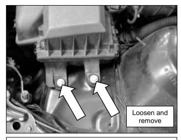
a. Loosen and remove the two bolts holding down the air box.
