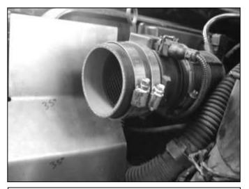
d. Attach coupler with supplied hose clamps.
