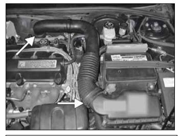
a. Loosen the hose clamps and disconnect the crankcase breather hose. Remove intake tubing.
