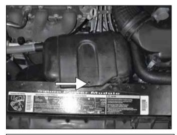
b. Remove the plastic clip from the resonator. Remove the resonator from the vehicle.
