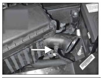
d. Unplug the IAT from the factory air box. Remove the air box from the vehicle.
