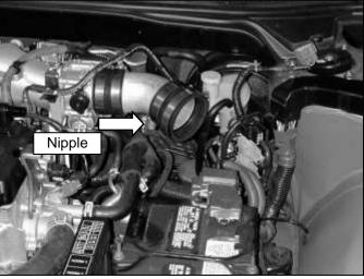
c. Install the upper intake pipe with the nipple pointing downward. Secure using the supplied couplers and hose clamps as shown.
