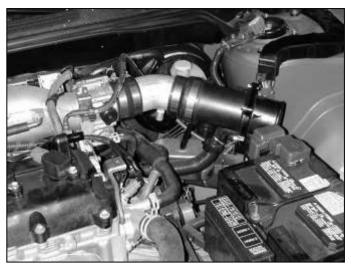
d. Install the MAF sensor assembly onto the upper intake pipe using the supplied coupler and hose clamps. Ensure the sensor connector is facing downward as shown. Reconnect the MAF sensor once the intake pipe is properly positioned.
