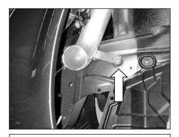
g. Secure the lower intake pipe to the rubber isolator using the supplied serrated nut and washer.
