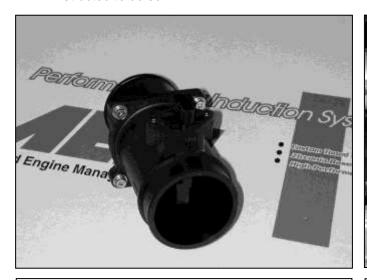
b. Bolt the adaptor to the MAF sensor using the factory bolts.
