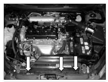
a. Remove the three plastic fasteners that secure the air scoop and then remove it.
