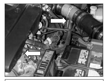
i. Install the included 5/6" breather hose onto the cam cover vent and the nipple on the upper intake pipe using the supplied 1" hose clamps.
