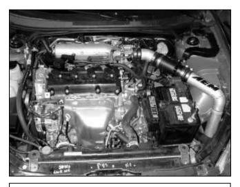
f. Install the middle intake pipe onto the MAF sensor adaptor. Loosely secure using the supplied coupler and hose clamps.
