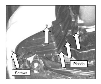
e. Remove the three plastic fasteners and two screws securing the inner fender. Move the fender liner to gain access to the inner front bumper.
