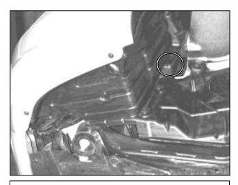
j. Install the fender liner and any hardware that was removed in step 2e. Some trimming of the fender liner may be necessary so that the rubber mount assembly installed in step 3g has adequate clearance.
