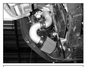
h. Install the air filter onto the longer leg of the lower intake pipe. Install the lower intake pipe assembly onto the middle intake pipe using the supplied coupler and hose clamps.
