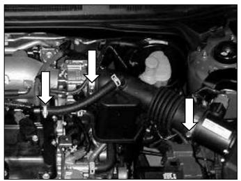
b. Squeeze stock hose clamp and remove hose from valve cover. Loosen the hose clamps as shown. Then remove the connector tube assembly.
