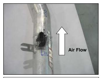
e. Insert the MAF sensor as shown.
