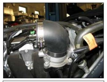
d. Attach the coupler at the throttle body as shown. Secure with the #44 hose clamps.
