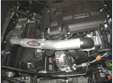
AEM® intake system installed
