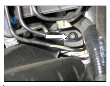
d. Loosen the inlet resonator tube mounting bolt located near the throttle body.
