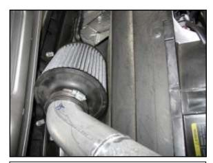
h. Attach the air filter element as shown and secure with the #48 hose clamp. Check for clearance against the radiator shroud. Attach filter sock to protect against the elements.
