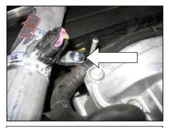
g. Align the bracket with the rubber mount. Secure with the M6 washer and M6 serrated nut. Reconnect the MAF sensor wire harness connector.
