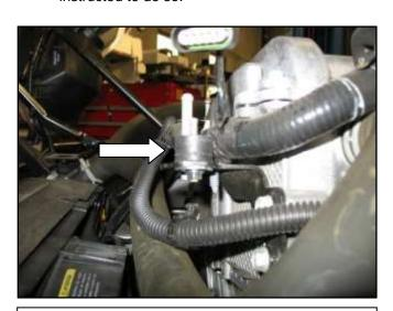
b. Install the supplied rubber mount. Secure the bottom of the rubber mount with the M6 washer and serrated nut in the hole left by the tree mount wire tie.
