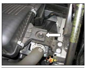
g. Loosen the remaining air box mounting bolt. Remove the air box from the engine bay, careful not to damage the hood.
