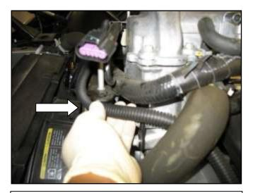
j. Remove the tree mount wire tie from the engine bracket.
