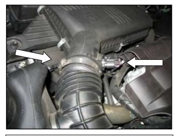
c. Loosen the hose clamp at the air box. Disconnect the mass air flow (MAF) sensor connector.
