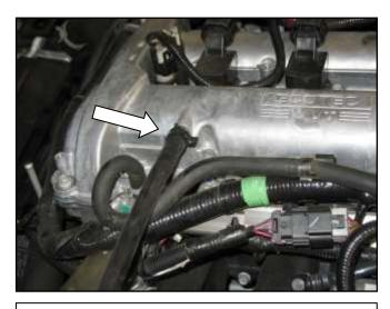
i. Remove the breather hose by unclasping the spring clamp. Both clamps will be reused.
