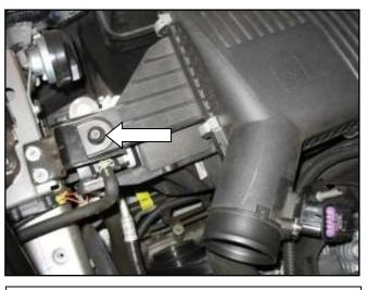
f. Loosen the air box mounting bolt.
