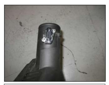
c. Remove the MAF sensor from the stock air box. The mounting screws will be reused.
