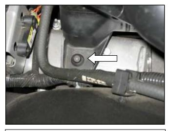
e. Loosen the remaining inlet resonator tube mounting bolt.
