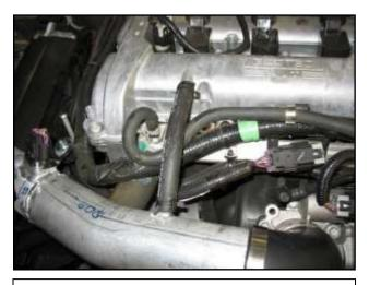
f. Insert the intake pipe into the coupler at the throttle body. Attach the supplied breather hose and secure with the factory spring clamps.
