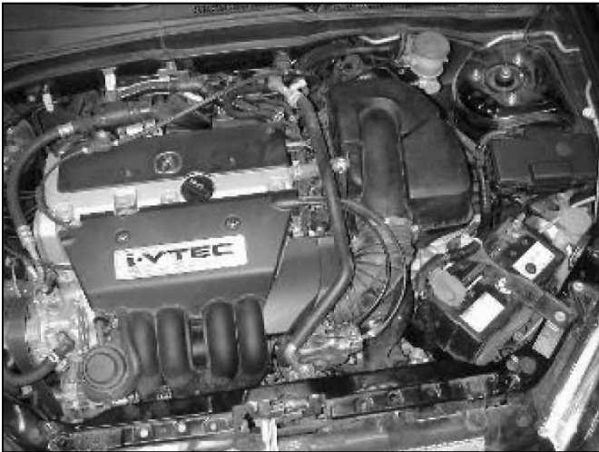
a. Factory air box system installed.
