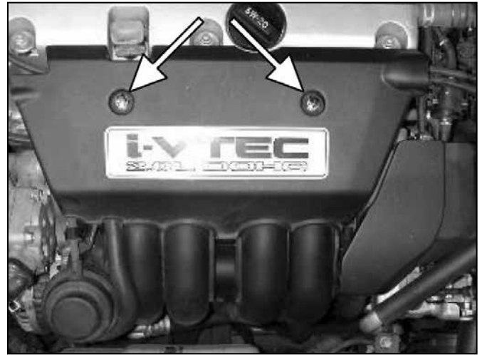
b. Remove the two bolts that secure the engine cover. Remove the engine cover.
