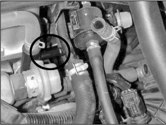
e. Pinch the clamp at the evaporative valve and pull the hose from the valve.
