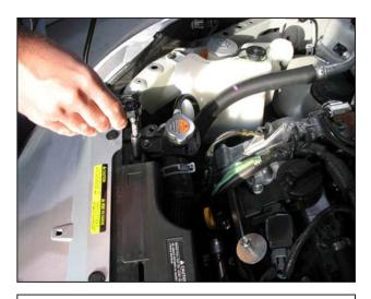
ag. Using the factory hex head bolt, secure the radiator trim panel in place.
