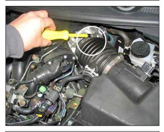
i. Loosen the hose clamp securing the inlet duct to the throttle body.
