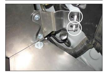
I. Remove the two nuts from the circled studs on the shock tower. Install the rear bracket as shown, use two M6 fender washers and M6-1 x 12mm hex head bolts to secure the bracket to the heat shield. Do not completely tighten the bolts.
