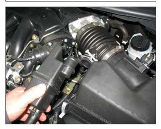
h. Remove the PCV resonator from the inlet duct.
