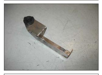
x. Install the rubber grommet onto the bracket as shown.
