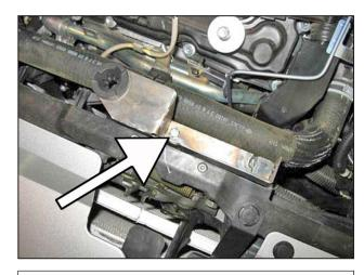
aa. Install the bracket with a M6-1x 12mm hex head bolt. Tighten the bolt enough to hold the bracket in place, but do not completely tighten.
