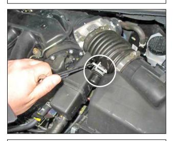
g. Loosen the clamp securing the positive crank case ventilation (PCV) resonator.
