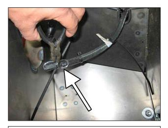
o. Cut the factory zip tie securing the wiring harness to the plastic push-in mounting tab.
