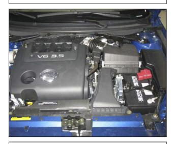
Factory air box system installed
