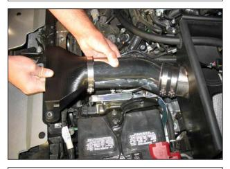
ab. Secure the air supply duct to the air supply scoop with a #9456 hose clamp. Install the assembly as shown.
