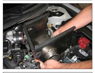
j. Install the heat shield in the vehicle, aligning the holes of the heat shield base with the aluminum mounts that were installed in steps 3d-3f.
