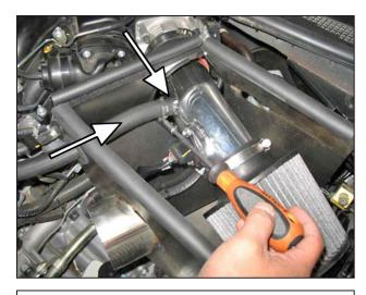
t. Insert the 5/8" I.D. PCV hose through the heat shield grommet and connect it to the intake pipe's nipple. Secure the PCV hose with a 1 1/16" hose clamp.
