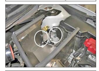
m. Place two M6 fender washers over the two shock tower studs. Reinstall the two nuts that were removed in the previous step. Completely tighten the two bolts and two nuts securing the bracket.
