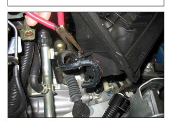
s. Remove the clip securing the ribber tube.
