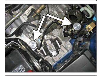
f. Ensure that the hardware securing the aluminum stands is completely tightened.
