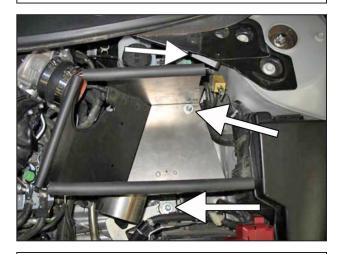
k. With the heat shield in place, install M6 fender washers and M6 nuts over each mounting stud. The black box mounted to the firewall near the heat shield may need to be adjusted for clearance. Carefully bend the black box's bracket towards the firewall to allow enough clearance.
