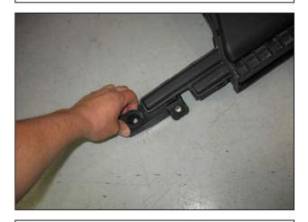
w. Remove the rubber grommet on the factory fresh air duct.
