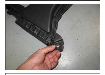
y. Remove the metal sleeve and rubber grommet from the factory fresh air duct.
