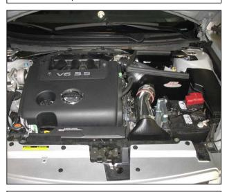
AEM® intake system installed
