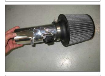
q. Remove the MAF sensor from the factory air box lid. Install the MAF sensor into the intake pipe with the factory screws. Install the air filter onto the intake pipe and secure it with a #9452 hose clamp.
