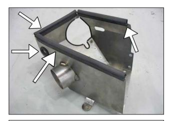
i. Install the edge trim onto the top edges of the heat shield and trim to fit. Install the rubber grommet in the heat shield hole as shown.
