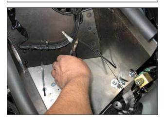
p. Route the MAF sensor wiring as shown and secure the wiring harness with the two zip ties. Trim the excess zip tie ends.
