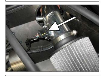
s. Plug in the MAF sensor harness connector to the MAF sensor
