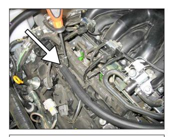
u. Connect the other end of the PCV hose to the port on the engine. Secure the PCV hose with a 1-1/16" hose clamp.
