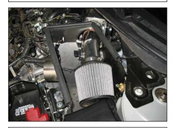
r. Install the intake pipe assembly as shown. Position for optimal clearance, ensuring that the assembly does not contact any surrounding parts. Secure the intake pipe to the coupler installed on the throttle body.
