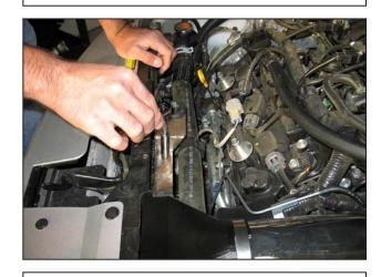
ae. Tighten the M6 hex head bolt securing the bracket.
