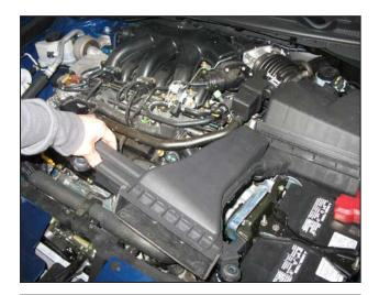
e. Remove the fresh air duct.
