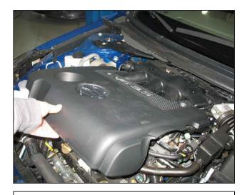
f. Remove the engine cover by pulling the cover upward at the front edge.
