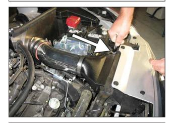
ad. Secure the air supply scoop with the factory hex head bolt.
