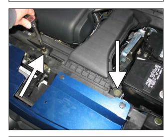
d. Loosen and remove the two hex head screws on the fresh air duct.
