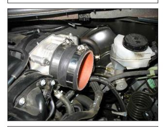
g. Install the 3.25" to 3.00" diameter hose adapter onto the throttle body. Secure the adpater in place with a #9452 hose clamp. Slide a #9448 hose clamp onto the smaller diameter side of the adapter hose.
