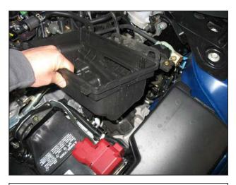
r. Remove the air box base by lifting upwards, this will require some effort because the base is secured in place with two rubber grommets on the bottom side.
