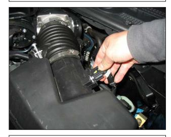
j. Unplug the Mass Air Flow (MAF) sensor harness connector from the sensor.
