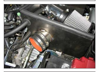
v. Install the 3.50" x 2" silicone coupler onto the heat shield inlet tube. Slide two #9456 hose clamps onto the silicone coupler.
