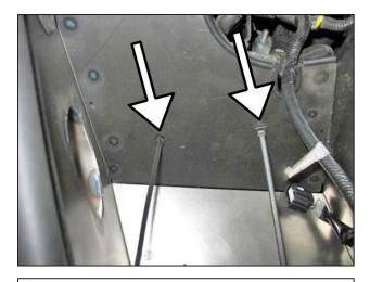
n. Install two push in zip ties on the inside wall of the heat shield. Route the MAF sensor wiring into the heat shield as shown.
