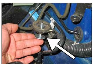
c. The hardware prepared in step 3b will slide through the factory grommets as shown. If the factory grommets are missing, check the bottom of the air box base or the engine bay as they may have fallen out when the air box was removed.
