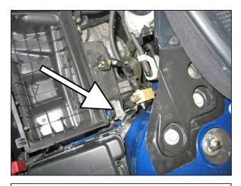
q. Remove the hex head screw securing the air box base.
