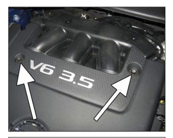
b. Loosen and remove the socket cap head screws on the engine cover.
