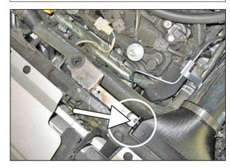
ac. Insert the nub of the air supply scoop into the hole of the bracket.
