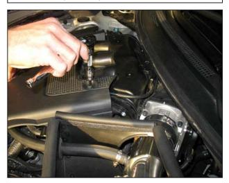
ai. Secure the engine cover with the hardware removed in step 2b.
