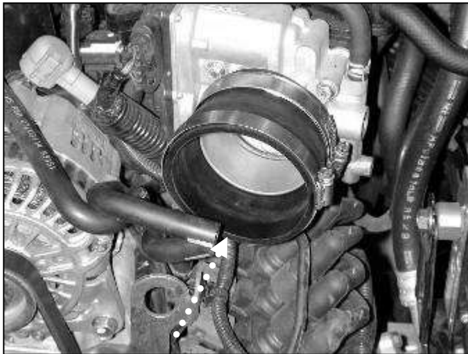
b. Attach the reducer coupler and secure with the provided #48 hose clamp.
