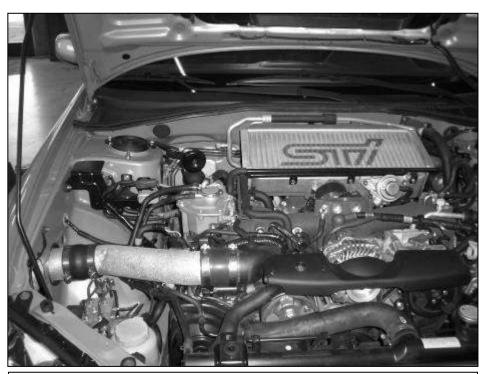
AEM® intake system installed.
